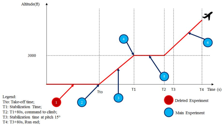
**Figure 3 - Flight Procedure**
