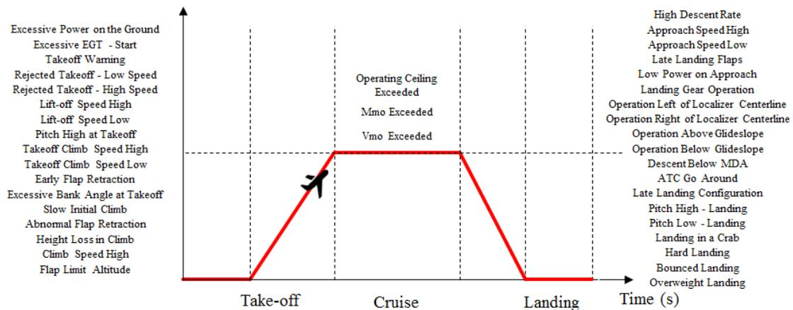
**Figure 2 – Flight phases and FOQA events**
