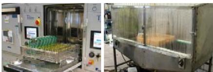
Fig 3. *Left*: Traditional cleaning equipment using Qlean water at Flextronics. *Right*: Demonstrator developed within IQ.
