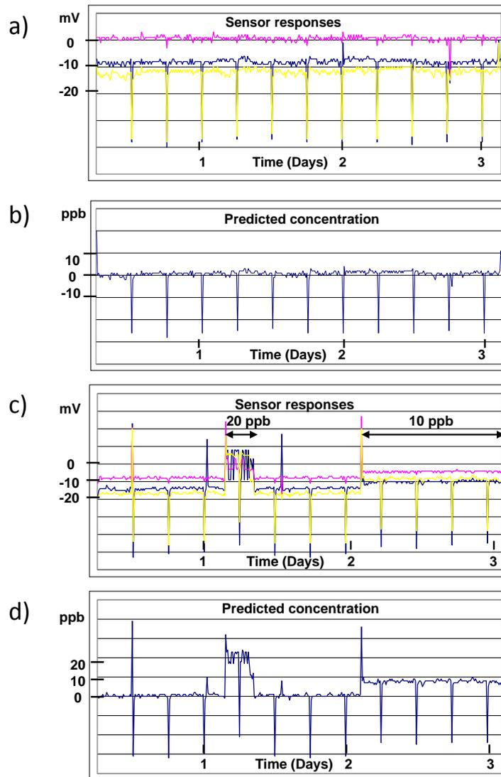
Fig. 3. Field measurements at the Görveln water works outside Stockholm, Sweden. a) Responses of the three gas sensors as a function of time. Every six hours a cleaning step is performed which induces a negative spike. b) Predicted diesel concentration from the sensor data in a). c) Sensor responses during addition of two different concentrations of diesel (10 and 20 ppb) as indicated by the arrows d) Predicted diesel concentration from the sensor data in c).
