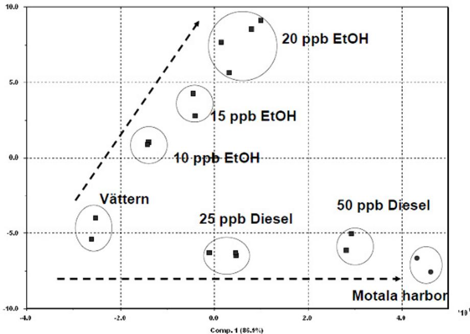
Fig. 2. PCA plot from lab measurements of water from the lake Vättern, Sweden, with different concentrations of diesel or ethanol (EtOH) added to the water. Also a sample of water from the harbor of the town Motala at the lake is included.
