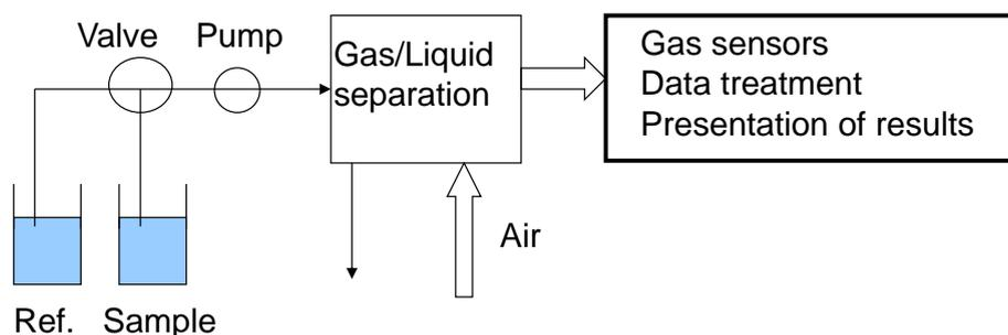
Fig. 1. A schematic illustration of the measurement setup.
