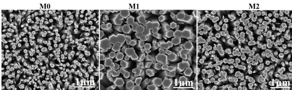
Fig. 1: SEM images of pure ZnO (M0) and Co-doped ZnO NRs as-synthesized using approaches M1 and M2, respectively.
