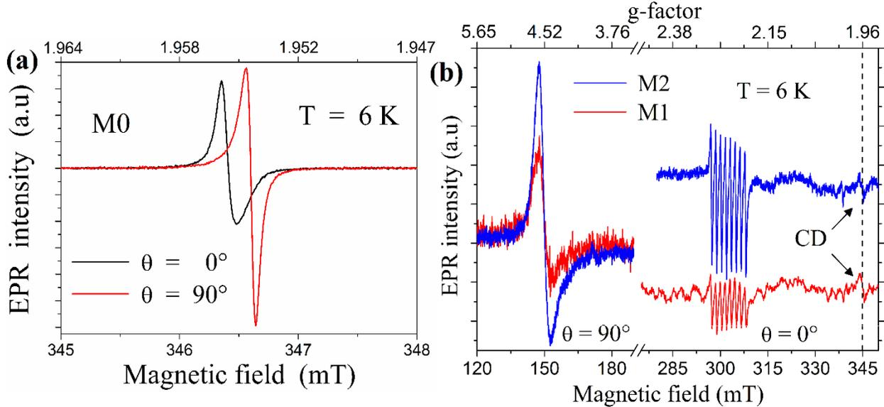
Fig. 3: (a) EPR spectra show anisotropy of the CD signal in the pure ZnO sample (M0). (b) EPR spectra of Co-doped ZnO NRs ( M1 and M2 ) for parallel ( $\theta = 0^\circ$ ) and perpendicular ( $\theta = 90^\circ$ ) orientation of magnetic field, recorded at  $T = 5$  K. The upper axis gives corresponding g factor values.
