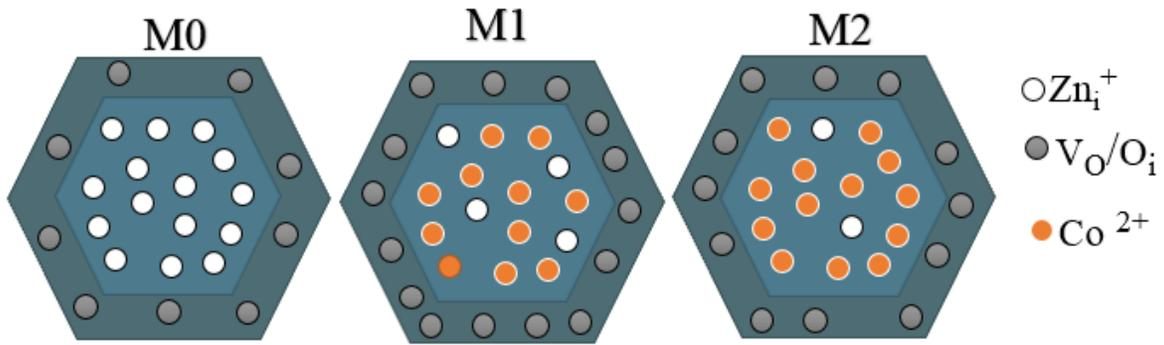
Fig. 5: Schematic illustration of the cross-sectional view of the as-synthesized pure ZnO and Co-doped ZnO NRs containing  $Zn_i^+$  as core-defect and oxygen vacancies/interstitials as surface defects, respectively.
