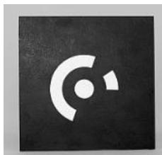
Figure 3.2.3. A 14-digit target tile, each tile is unique.
