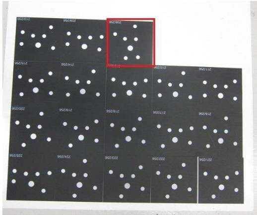
Figure 3.2.1. A sheet of ANCO reference target stickers.
