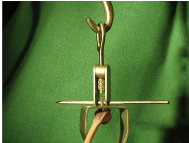
*Figure 2. Experimental set up for pullout measurements. The metal hook was connected to a force transducer. The metal plate, through which the screw head points out, was connected to a stepping motor moving down at a speed of 0.2 mm/s.*
