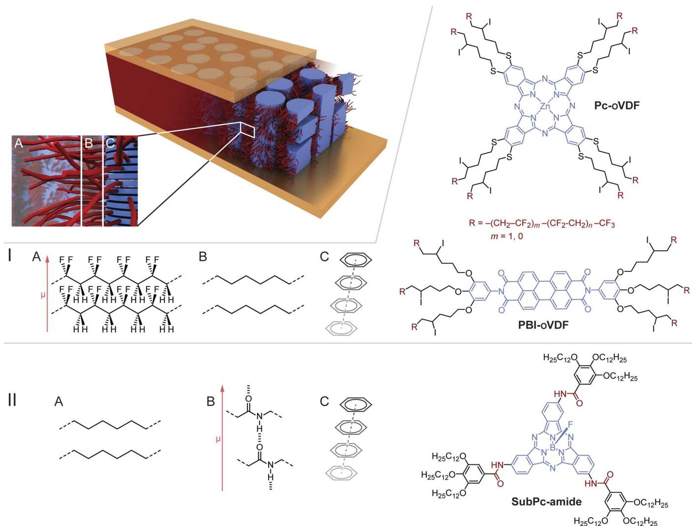
**Fig. 1. A cartoon of the devices studied and the chemical structure of the investigated oFESC compounds and their supramolecular organization.** Semiconducting cores are shown in blue, and dipolar side groups are shown in red. (I) Structures of PBI-oVDF and Pc-oVDF. (II) Structure of SubPc-amide. For details of the synthesis and characterization, see the Supplementary Materials.
