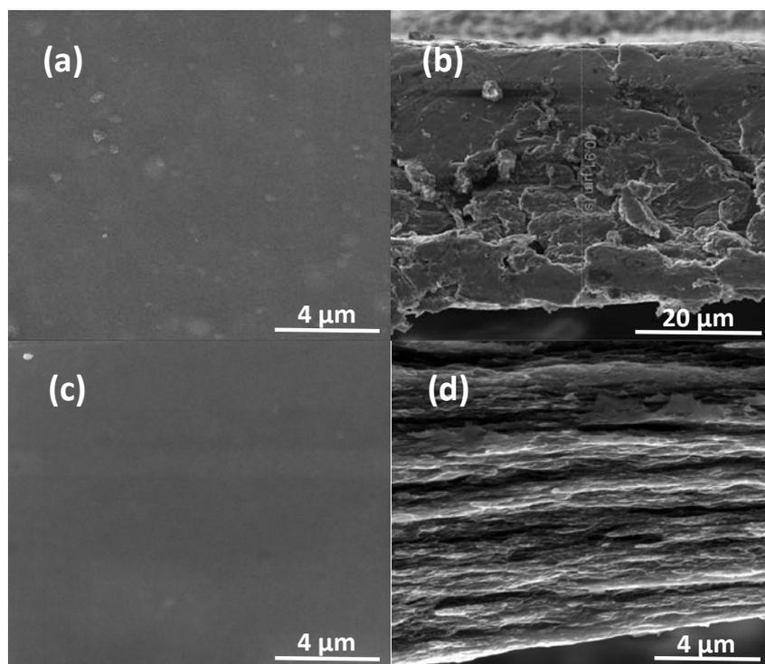
**Figure S5** SEM photographs of surface (a, c) and cross-section (b, d) of free standing PEDOT:PSS films before and after treated with concentrated sulfuric acid.
