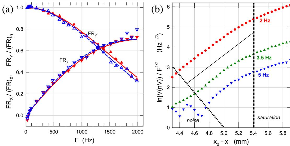
**Figure 2** (a) Experimental data used to determine the through-plane diffusivity: frequency dependence of the photothermal signals in-phase ( $R_X$ ) and in quadrature ( $R_Y$ ) with the input
