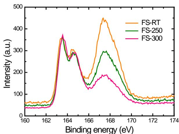
**Figure S3** XPS characterization of FS-PEDOT:PSS samples treated for 10 minutes in glove box at room temperature, 250 and 300°C, respectively.
