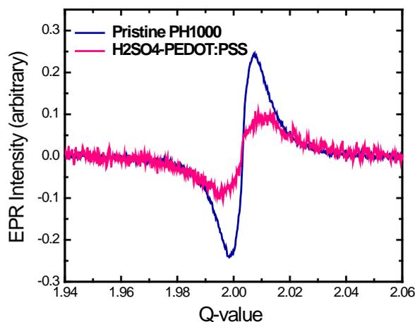
**Figure S1** EPR spectra of pristine PEDOT:PSS film and concentrated sulfuric acid treated PEDOT:PSS film. The films were fabricated by spincoating method on thin-glass substrate. As for the H<sub>2</sub>SO<sub>4</sub>-PEDOT:PSS film, it was spincoated from the PEDOT:PSS paste and then treated by concentrated sulfuric acid for 10 min at room temperature.
