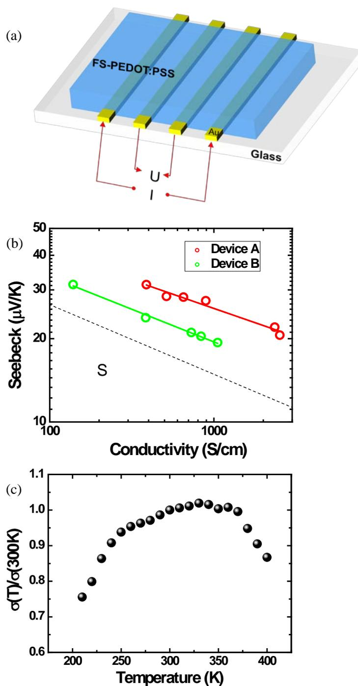
**Figure 1** (a) Device structure of  $\sigma$  and  $S$  measurement, channel width between gold electrodes is 1 mm. (b) The relationship between  $\sigma$  and  $S$  of FS-PEDOT:PSS films under different doping level with TDAE, the dashed line is the indication of  $S \sim \sigma^{1/4}$ . (c) Temperature dependent  $\sigma$  of FS-PEDOT:PSS in a temperature range from 200 to 400K.
