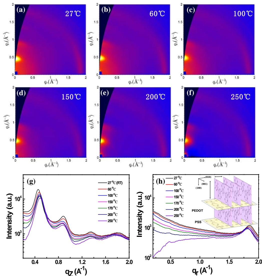
**Figure 5** 2D GIWAXS patterns of the FS-PEDOT:PSS film (a) without annealing and (b-f) in-situ annealed with increasing temperatures. GIWAXS intensity profiles along the (g) out-of-plane and (h) in-plane (Inset: Illustration of crystalline FS-PEDOT:PSS) directions.
