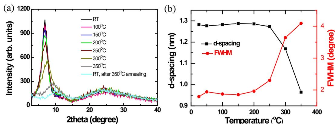
**Figure 4** (a) Temperature-dependent XRD characteristics of FS-PEDOT:PSS at different temperature (room temperature (RT) to 350 °C). (b) The statistics of temperature-dependent spacing (d-spacing) and full-width at half-maximum (FWHM).
