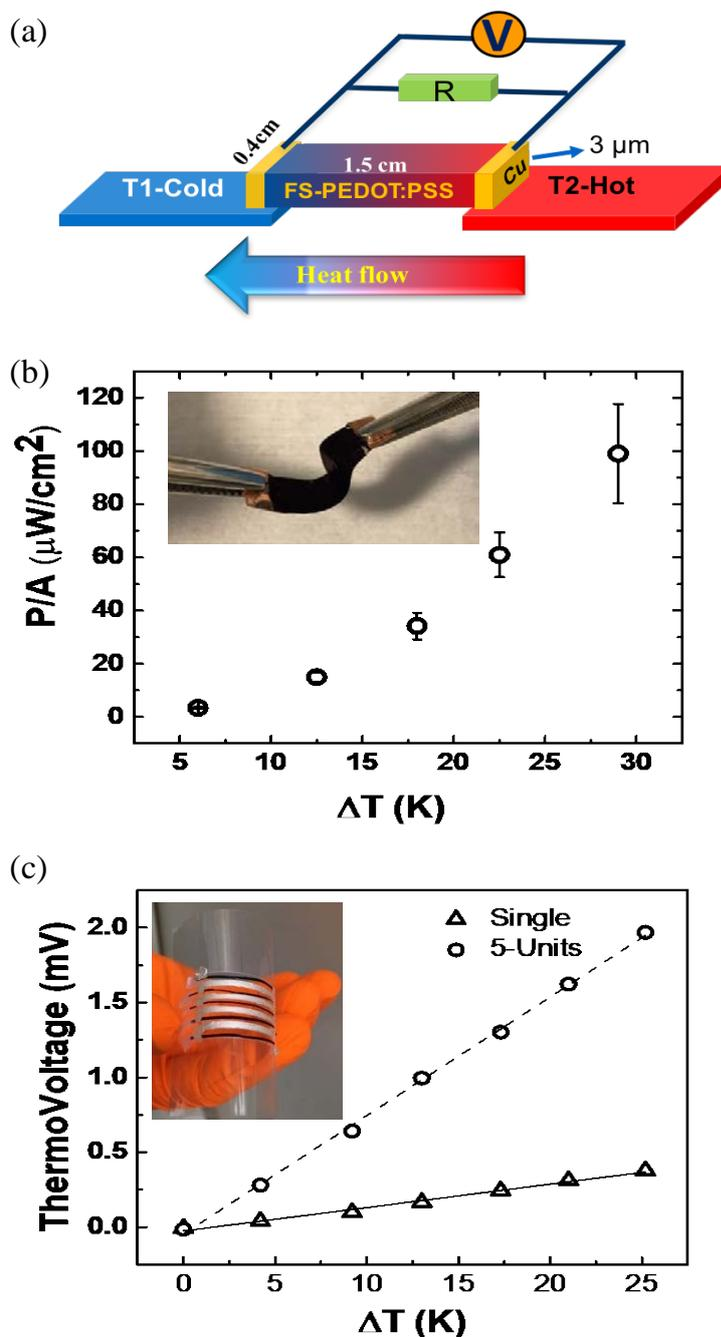
**Figure 3** (a) A free standing TE device based on FS-PEDOT:PSS film. (b) Power output per cross section area of the free standing TE device. The inset is a photo-picture of the free standing TEG device. The length of the device between the heat and cold source is  $L=1.5$  cm, film width is 0.4 cm
