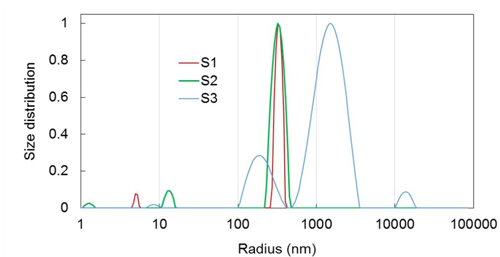
**Figure S4** DLS measurement of pristine PH1000 (S1), PH1000 + 5% EG (S2) and PEDOT:PSS paste (S3).
