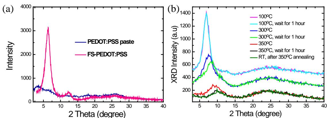
**Figure S2** (a) XRD measurement of free standing PEDOT:PSS films before (PEDOT:PSS paste) and after (FS-PEDOT:PSS) concentrated sulfuric acid treated. (b) Time-dependent XRD of FS-PEDOT:PSS film at different temperatures of 100, 300 and 350°C.
