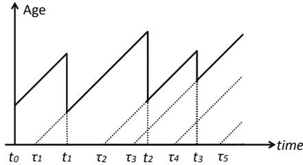
Fig. 2. Age evolution for a source. The  $i$ th packet with time stamp  $\tau_i$  is received by the destination at  $t_i$ . The age at  $t_i$  equals  $t_i - \tau_i$ . The age increases linearly if no packet is received.
