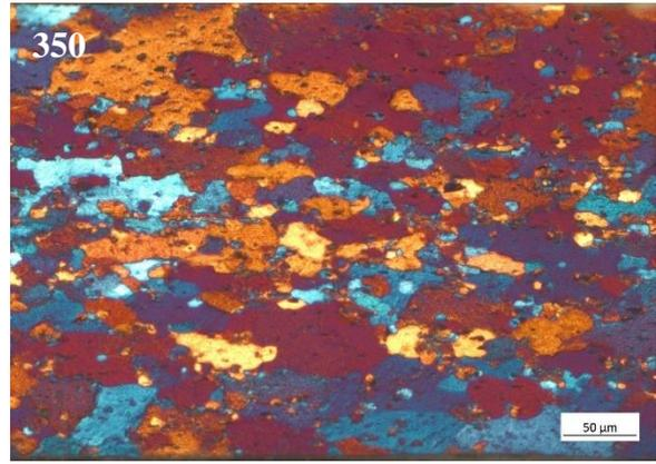
*Figure 4.12: Longitudinal images of cross section of unhomogenised samples.*
