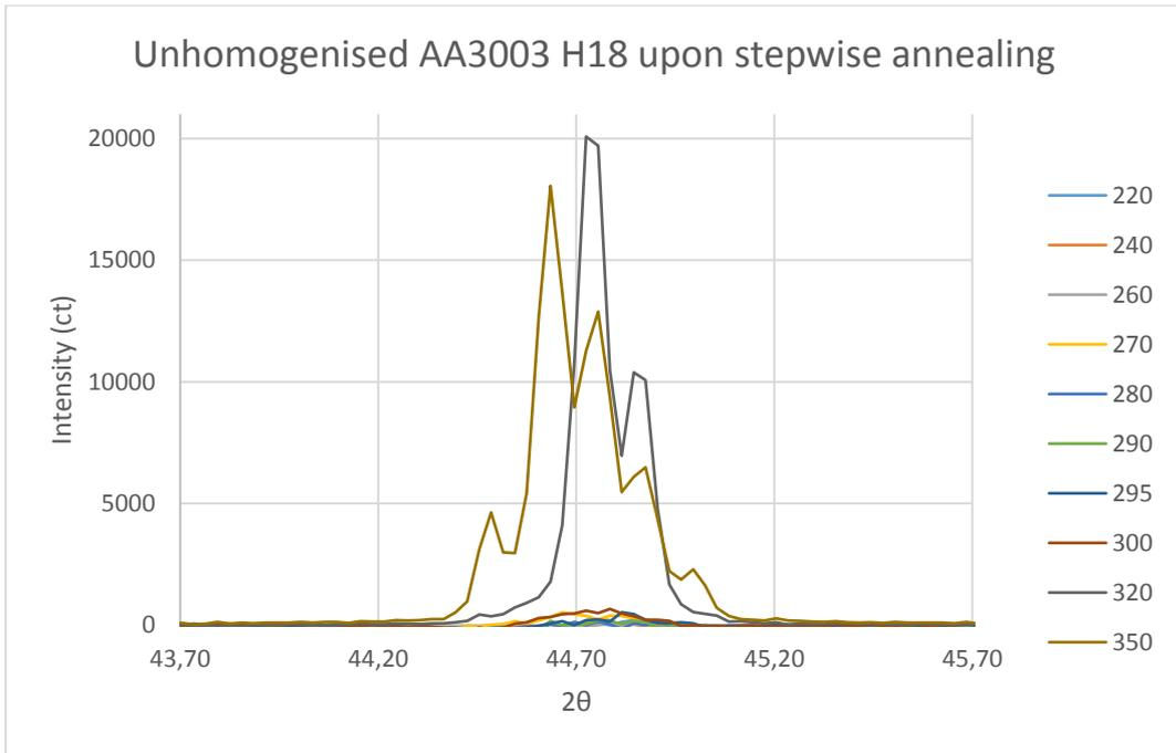
Figure 4.6: Intensity change of Al (200) in unhomogenised AA3003 H18 upon stepwise annealing.
