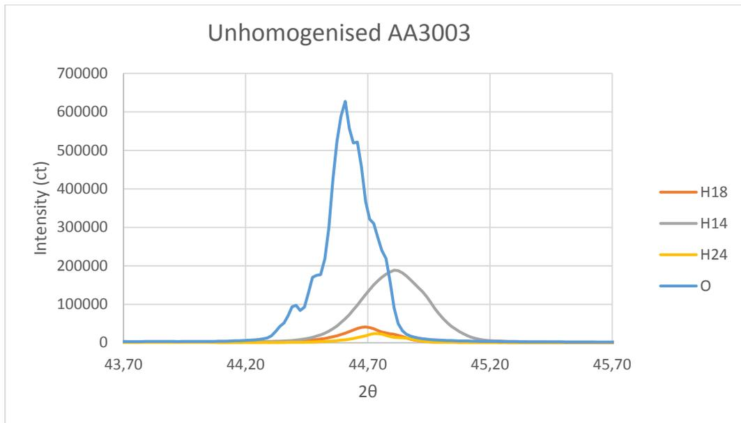
Figure 4.4: Close-up of peak Al (200) in unhomogenised AA3003.
