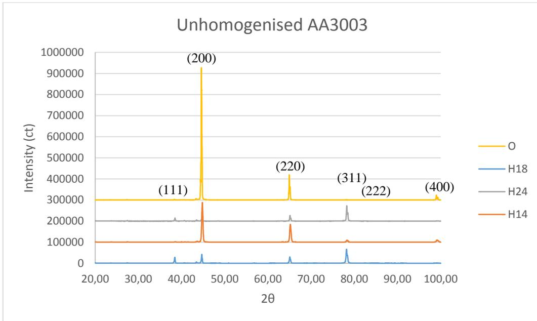
Figure 4.2: Measured diffractogram of unhomogenised AA3003 at different temps.
