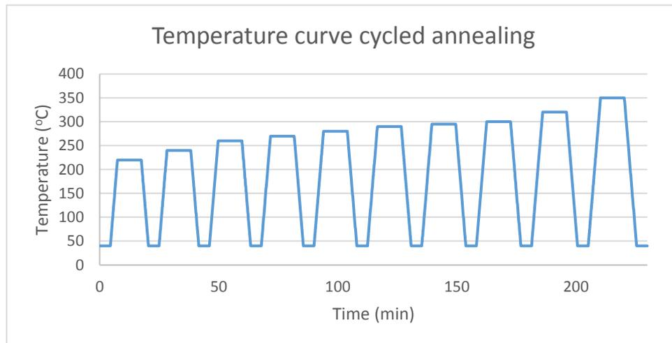
Figure 3.2: Temperature cycles used during annealing experiments.
