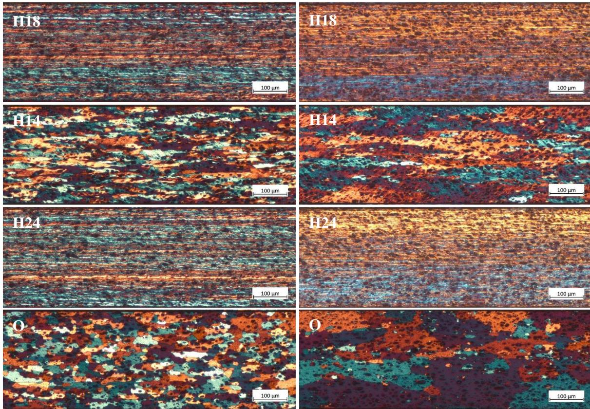
*Figure 2.2: LOM images of AA3003 at different tempers, homogenized to the left and unhomogenized to the right.*
