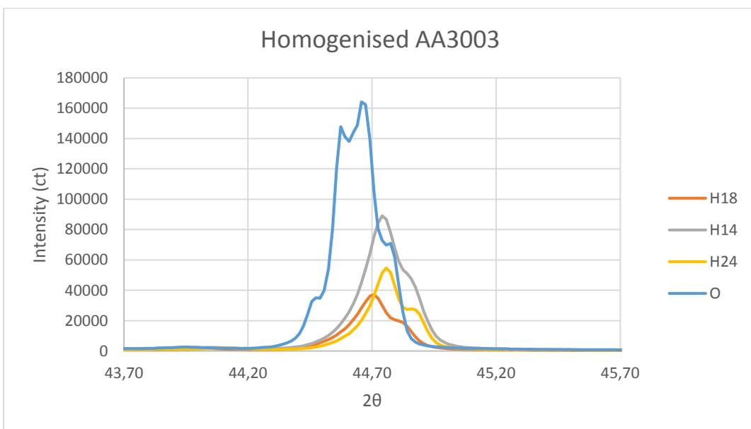
Figure 4.3: Close-up of peak Al (200) in homogenised AA3003.
