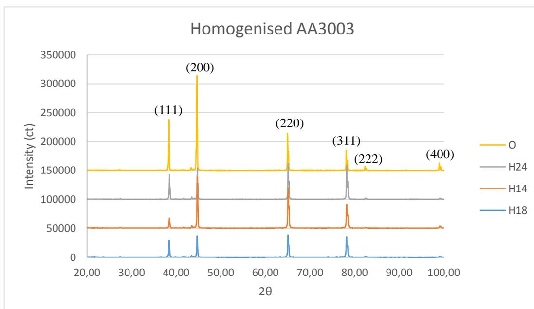
*Figure 4.1: Measured diffractogram of homogenised AA3003 at different tempers.*
