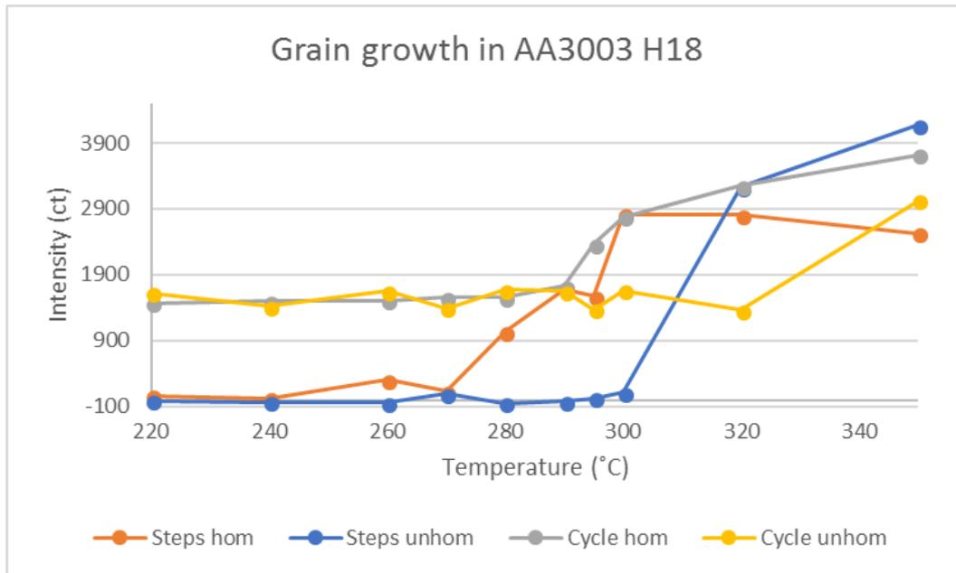
Figure 4.10: Summarised intensity beneath Al (200) at different temperatures.
