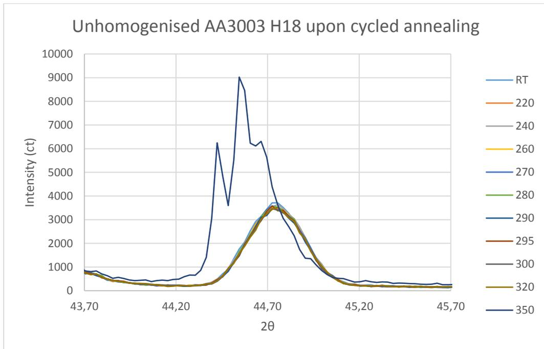
Figure 4.8: Intensity of Al (200) in unhomogenised AA3003 H18 during cycled annealing.
