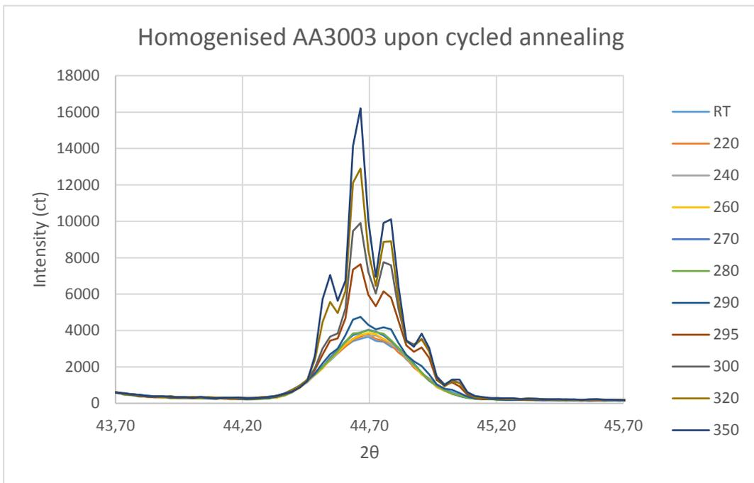
Figure 4.7: Intensity of Al (200) in homogenised AA3003 H18 during cycled annealing.
