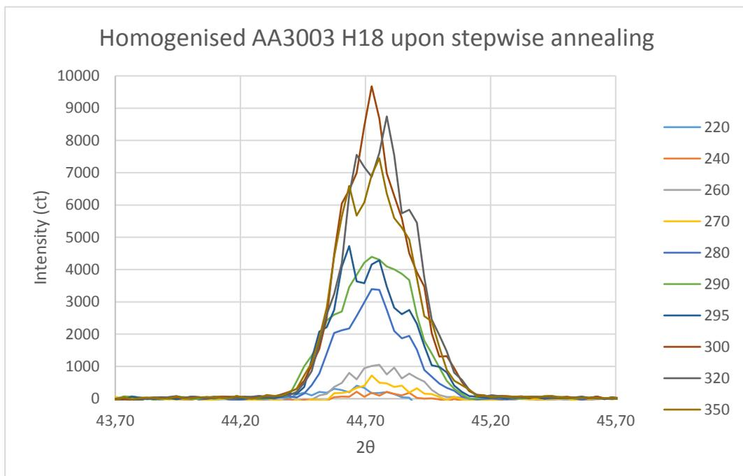
Figure 4.5: Intensity change of Al (200) in homogenised AA3003 H18 upon stepwise annealing.
