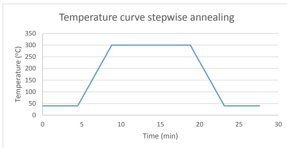
Figure 3.1: Example of the temperature curve used during stepwise annealing, here up to 300 °C.
