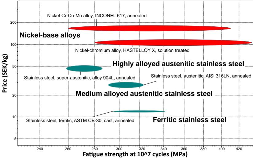
Figure 1: Difference in price [SEK/kg] vs. fatigue strength (max stress to survive  $10^7$  cycles, RT,  $R=-1$ ), for power plant materials (From CES EduPack 2018).
