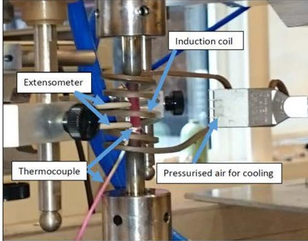
Figure 4: The setup for the TMF test machine.
