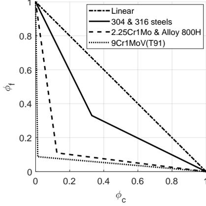
Figure 3: Example of a creep-fatigue damage envelope (interaction diagram) re-plotted from ASME Code [32] with axes interchanged (same as in [33]).
