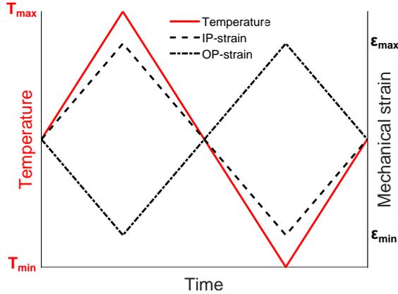
Figure 2: The most common TMF test cycles, in-phase (IP) and out-of-phase (OP).
