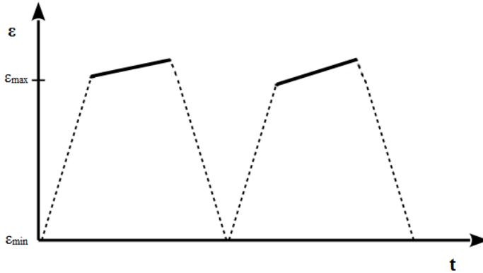
Figure 5: Sketch of the creep-LCF test cycle, strain vs. time
