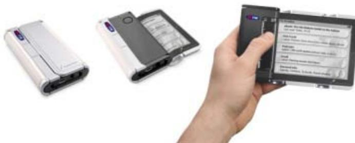
Figure 1. A mobile device rollable polymer display for reading personal information, newspapers and books (by Polymervision, [www.polymervision.com](http://www.polymervision.com)). The display type is based on rollable organic thin-film transistor backplane with electrophoretic front plane with a total thickness of about 0.1 mm, equal to the thickness of everyday paper.
