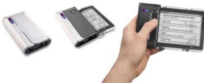
Figure 1. A mobile device rollable polymer display for reading personal information, newspapers and books (by Polymervision, www.polymervision.com ). The display type is based on rollable organic thin-film transistor backplane with electrophoretic front plane with a total thickness of about 0.1 mm, equal to the thickness of everyday paper.
