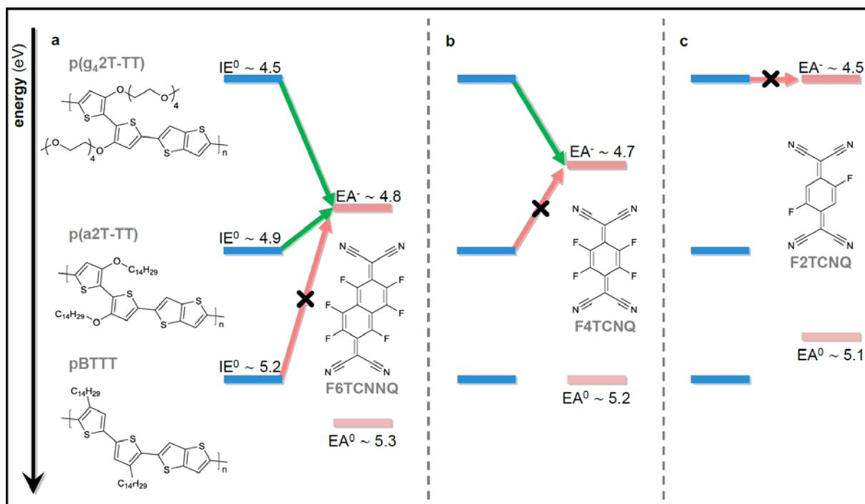
**Fig. 2 | Energy diagram summarising the formation of dopant dianions.** Doping of p(g<sub>4</sub>2T-TT), p(a<sub>2</sub>T-TT) and pBTTT with **a**, F6TCNNQ, **b**, F4TCNQ, and **c**, F2TCNQ; IE<sup>0</sup> of the polymers as well as EA<sup>0</sup> and EA<sup>-</sup> of the dopants were measured with cyclic voltammetry (CV) (Supplementary Figs. 5 and 6). Green (red) arrows indicate where electron transfer from the polymer to the dopant anion is observed (absent).
