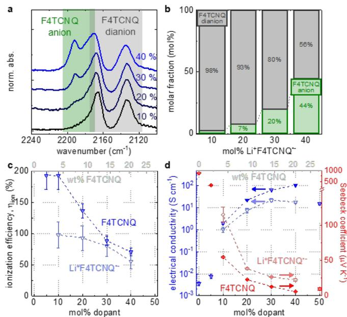
**Fig. 4 | Comparison of doping of p(g<sub>4</sub>2T-TT) with F4TCNQ and Li<sup>+</sup>F4TCNQ<sup>-</sup>.** **a**, Solid-state FTIR absorption spectra of p(g<sub>4</sub>2T-TT) doped with 10, 20, 30 and 40 mol% Li<sup>+</sup>F4TCNQ<sup>-</sup> per repeat unit, and **b**, molar fractions of F4TCNQ anion (green) and dianion (grey) in the corresponding films determined from the relative FTIR intensities of anions
