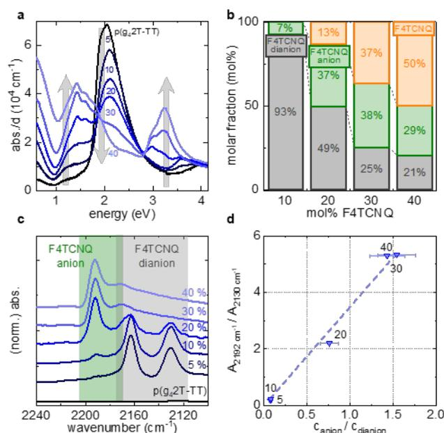
**Fig. 3 | Amount of neutral, anionic and dianionic F4TCNQ in doped p(g<sub>4</sub>2T-TT) films.**
