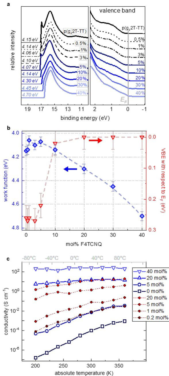
**Fig. 5 | Work function and temperature-dependent conductivity of F4TCNQ doped p(g<sub>4</sub>2T-TT).** **a**, UPS spectra of neat p(g<sub>4</sub>2T-TT) and doped with increasing amounts of F4TCNQ showing the photoemission cut-off (left) and the valence band region (right). **b**,
