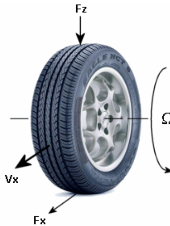
Figure 2.12: The forces on the tire used in Pacejka's magic formula,[8].
