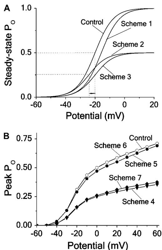
FIGURE 3 Effects of different block mechanisms on activation curves. Computed steady-state and peak open probability ( $P_O$ ) plotted against potential for the different blocking schemes (see Figs. 1 and 2), assuming  $K_d$  concentration and intermediate blocking rate. (A) Noninactivating channels, Schemes 1–3 (see Appendix A). (B) Inactivating channels, Schemes 4–7.
