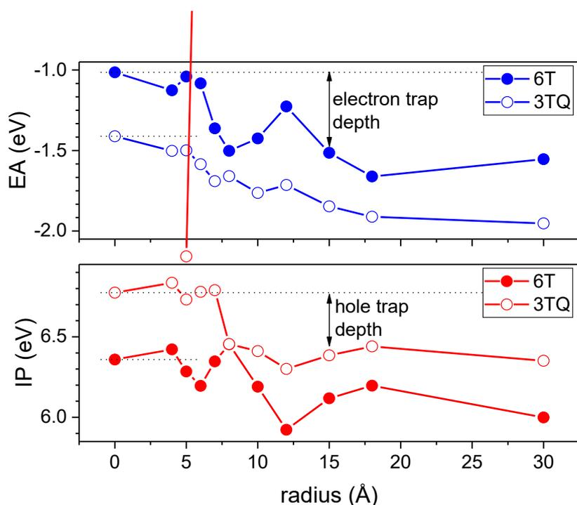
**Figure 5 | Evolution of IP and EA with water nanodroplet size.** Electron affinity (EA, blue) and ionization potential (IP, red) as calculated by QM/MM for a 6T (solid lines) or a 6TQ (dashed lines) oligomer with a nano-droplet of water of the indicated radius at its center. Zero radius corresponds to vacuum.
