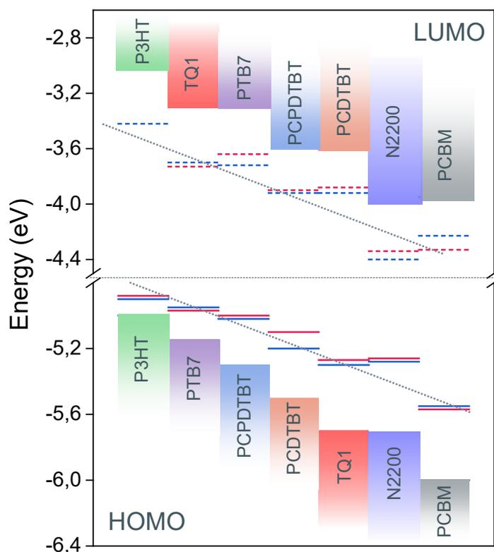
**Figure 3 | Electron and hole trap energies.** Hole (solid lines) and electron (dashed lines) trap energies in relation to HOMO (shaded area on bottom) and LUMO (top) energy levels for the investigated range of organic materials. Trap energies determined by slope- and JV-fitting are shown as red and blue lines, respectively. The thin black dotted lines are guides to the eye.
