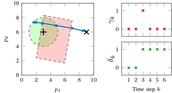
Fig. 4. The setup is the same as in Fig. 3, but the weight of stealth has been given a lower value ( $w_{\mathcal{I}} = 1, w_P = 0.01, w_{x,u} = 0.01$ ). Left: Computed path for the mobile robot. Upper right: Binary variables indicating whether or not the adversarial sensor obtains measurements. Lower right: Binary variables indicating whether or not the mobile robot obtains measurements.
