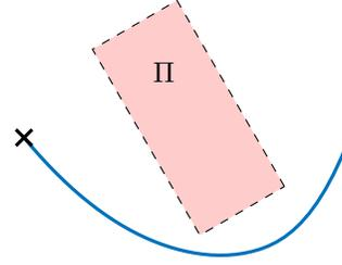
Fig. 2. A mobile robot is being tracked by an adversarial sensor, that obtains measurements if the mobile robot is within its sensing region (red area). The problem is to find a stealthy path for the mobile robot; the objective is to minimize the adversarial sensor's tracking performance.
