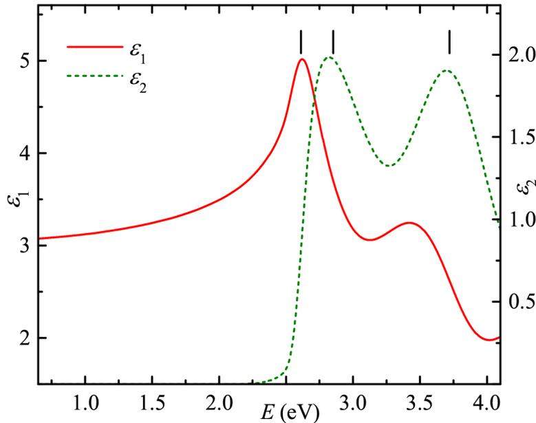
**Fig. 3.** Real  $\varepsilon_1$  (solid red line) and imaginary  $\varepsilon_2$  part (dotted green line) of the model dielectric function given in Eqn. (1) using the best-fit model parameters summarized in Table 1. The transition energies for the Tauc-Lorentz and the Gaussian oscillators are indicated as vertical lines.
