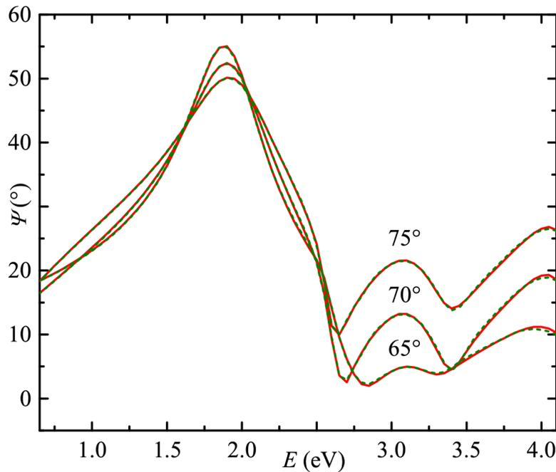
**Fig. 1.** Experimental (green dashed line) and best-model (red solid line)  $\Psi$ -spectra for the Si(bzimp)<sub>2</sub> sample measured at three different angles of incidence  $\Phi_a = 65^\circ, 70^\circ,$  and  $75^\circ$  in spectral range from 0.65 eV to 4.1 eV.
