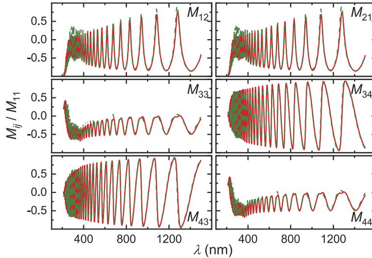
**Fig. 2.** Experimental (green dashed lines) and best-model calculated (red solid lines) Mueller matrix spectra of the two-photon polymerized IP-L sample with a nominal thickness of 2900 nm for the spectral range from 210 nm to 1500 nm. The angle of incidence was  $\Phi_a = 65^\circ$ . The data for the sample with a nominal thickness of 4300 nm is omitted here for clarity, but shows also an excellent agreement between experimental and best-model calculated line shapes.
