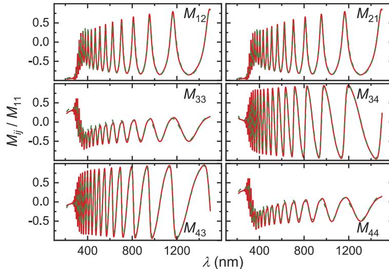
**Fig. 1.** Experimental (green dashed lines) and best-model calculated (red solid lines) Mueller matrix spectra of the two-photon polymerized IP-Dip sample with a nominal thickness of 2100 nm for the spectral range from 210 nm to 1500 nm. The angle of incidence was  $\Phi_a = 65^\circ$ . The data for the sample with a nominal thickness of 3500 nm is omitted here for clarity, but shows also excellent agreement between experimental and best-model calculated line shapes.
