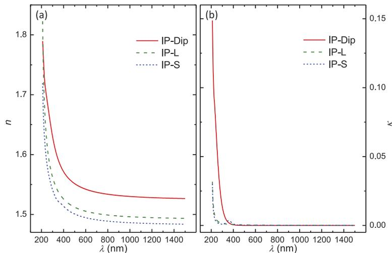
**Fig. 7.** The best-fit model refractive indices  $n$  and extinction coefficients  $\kappa$  for the two-photon polymerized IP-Dip, IP-L, and IP-S are reproduced in panel (a) and (b), respectively, for a direct comparison.
