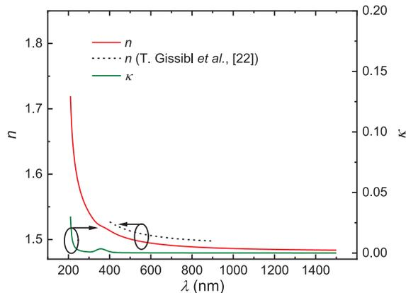
**Fig. 6.** Same as Fig. 4 but for IP-S, which can be described using two oscillators with Lorentz and Gaussian broadening. The best-model parameters are summarized in Table 1. In addition to the sharp absorption onset below 300 nm, a small absorption band at 358 nm can be observed. The refractive index of single-photon, UV-cured IP-S (black dotted line) reported by T. Gissibl *et al.* is shown for comparison [22].
