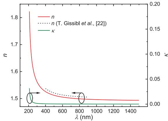
**Fig. 5.** Same as Fig. 4 but for IP-L. IP-L is characterized by a sharp absorption onset which can be described by a single Lorentz oscillator. The best-model parameters are summarized in Table 1. The refractive index of single-photon polymerized IP-L (black dotted line) reported by T. Gissibl *et al.* is shown for comparison [22].
