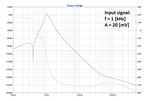
Figure 3.14: LTSpice simulation of filter with signal input frequency 1kHz and filter clock set to 10kHz
