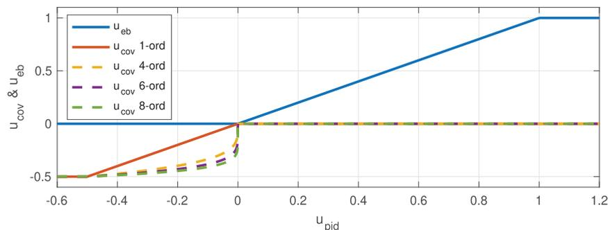
**Figure 5.** Examples of how the shape of the nonlinear compensator changes the COV control characteristics and how it depends on the order of the root.
