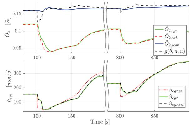
**Figure 7.** Oxygen Dynamics and EGR molar flows during the two first engine speed steps from Figure 6.
