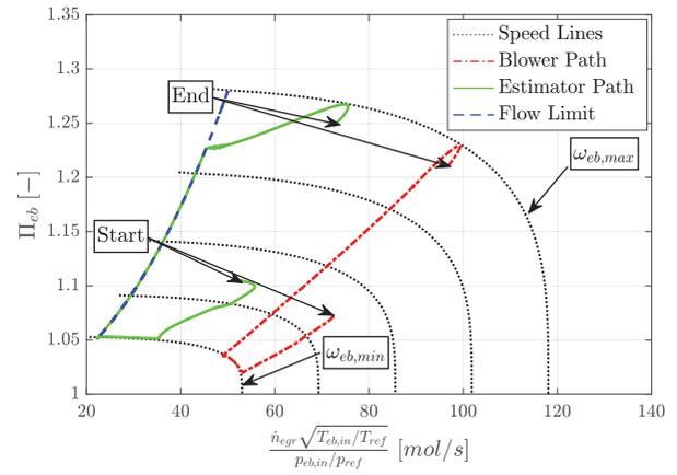
**Figure 9.** Real blower and flow estimator operating paths in the pressure ratio vs corrected molar flow plane. It corresponds to the  $p_{eb,in}$  3% ↓ case from Figure 8.
