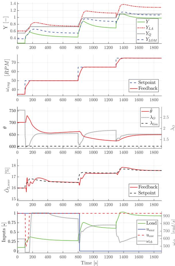
**Figure 6.** EGR and fuel controller performance during three consecutive engine speed steps.
