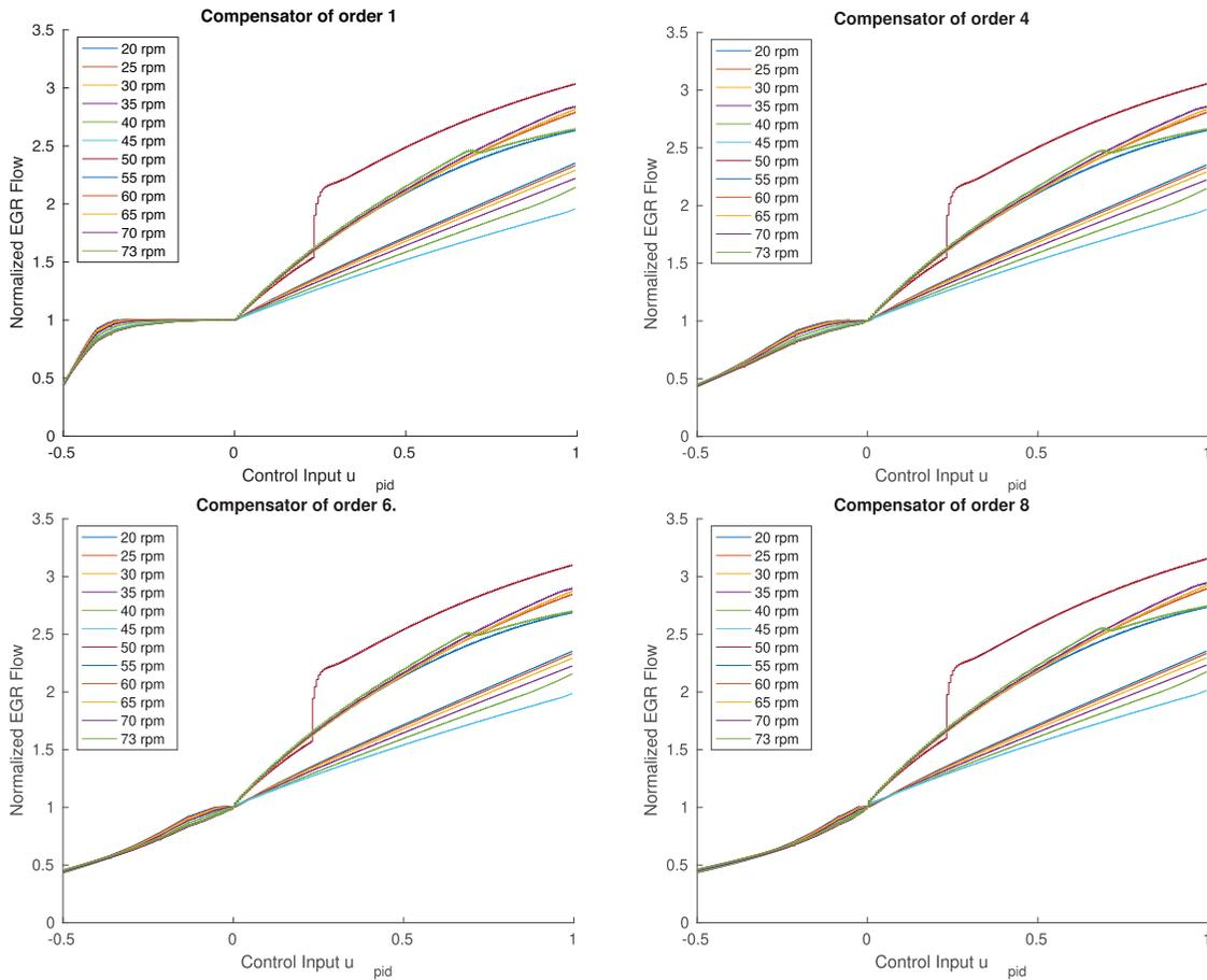
**Figure 4.** Example of nonlinear connection between achieved EGR-flow and control action  $u_{pid}$ . The **top left** describes the standard connection between the PID output and the normalised EGR. The other plots display what happens when the control action for the COV is changed using a non linear transformation defined in (13).
