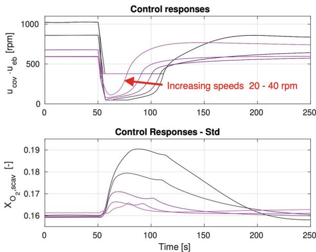
**Figure 13.** Response in Scavenge receiver oxygen concentration for the 5 steps at lowest speeds where the COV valve is active during the steps. This is for the standard controller without the actuator compensation. A bump is seen in the  $O_2$  responses during the decay phase, this comes from the phase when the COV actuator traverses the flat region for negative  $u_{pid}$  the left in the top left plot of Figure 4.
