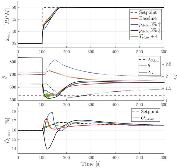
**Figure 8.** Low load speed step results for disturbances in the inlet pressure of the EGR flow estimator and noise added to the inlet temperature of the EGR blower.
