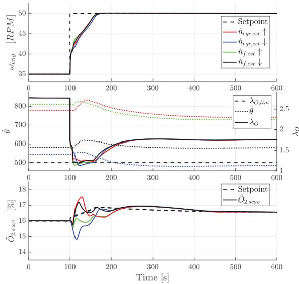
**Figure 10.** Low load speed step results for under and overestimation of EGR and fuel flows in the EGR controller.
