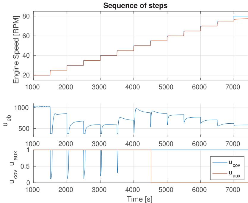
**Figure 11.** A sequence of steps in reference engine speed that ramps over the engine speed range with 5 RPM changes each time. The **top** plot shows the engine speed. The **mid** plot shows the EGR blower speed. The **bottom** plot shows the COV valve operation and the auxiliary blower. It is in the lower speed range where the  $u_{cov}$  becomes active, especially the first 5 steps cause the COV valve to close. These will be studied in more detail later.
