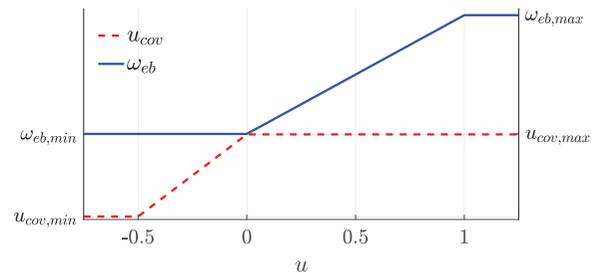
**Figure 3.** Split-range control diagram of the two actuator outputs depending on the PI controller output.
