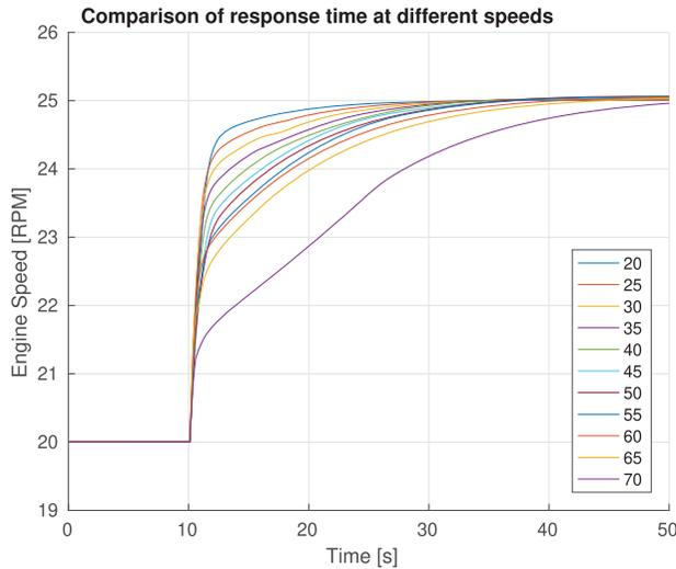
**Figure 12.** Speed steps from Figure 11 adjusted to make comparisons easy, by subtracting an offset so all start at 20 RPM. The response time for the engine speed increases with engine (and ship) speed.
