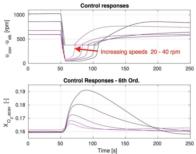
**Figure 14.** Response in Scavenge receiver oxygen concentration for the 5 steps at lowest speeds where the COV valve is active during the steps. This is for the nonlinear controller of order 6.
