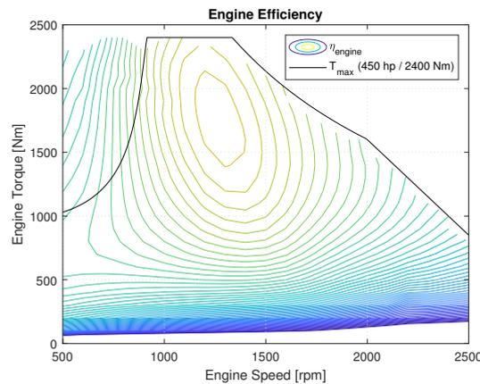
**Figure 2.** The stationary engine map for the MVEM. The maximum torque is set to 2400 Nm, the stationary air–fuel ratio limits the output torque to between 500 and 900 rpm, the maximum power is set to 450 hp and a high rpm cut-off is imposed at 2000 rpm. The diesel engine model’s maximum efficiency is 46%.
