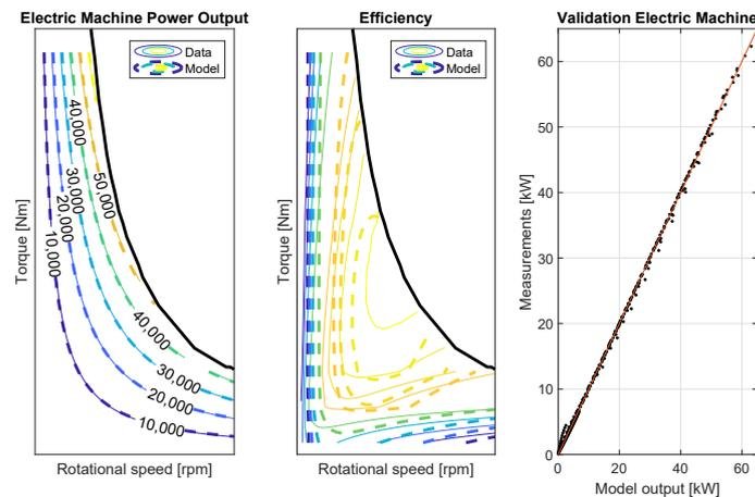
**Figure 4.** Electric motor power output and efficiency, and a comparison of the model's power output and the measured power output. Note that the highest efficiency island is not captured by the model.
