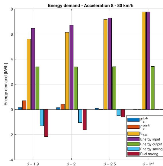
**Figure 14.** Consumed energy for different values of  $\beta$  during an acceleration from 8 to 80 km/h. The “Energy input” bar is the sum of the electrical energy and the diesel fuel. The “Energy output” bar is the work delivered to the engine main shaft. “Fuel saving” and “Energy saving” bars are relative to the minimum fuel solution ( $\beta = \text{inf}$ ).
