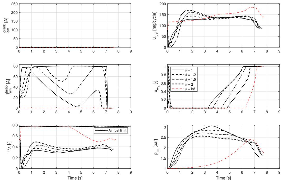
**Figure 8.** Controls, fuel-air ratio and intake manifold pressure, when the E-turbo is used to support the engine during the acceleration.
