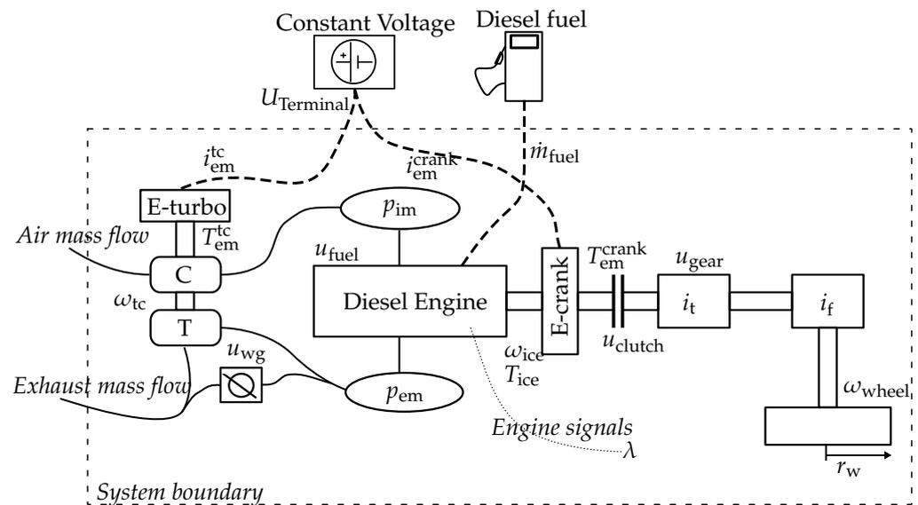
**Figure 1.** Terminology used to describe the diesel engine and the electric motors.
