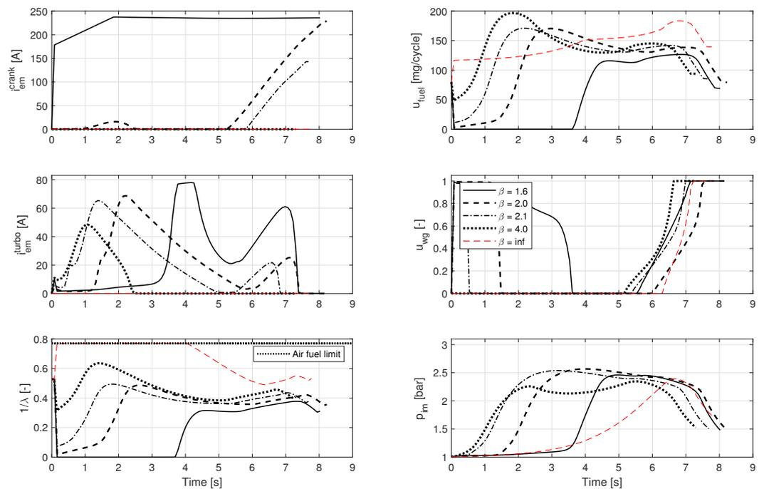
**Figure 12.** Controls, fuel-air ratio and intake manifold pressure during the acceleration when the engine is supported by both E-crank and E-turbo.
