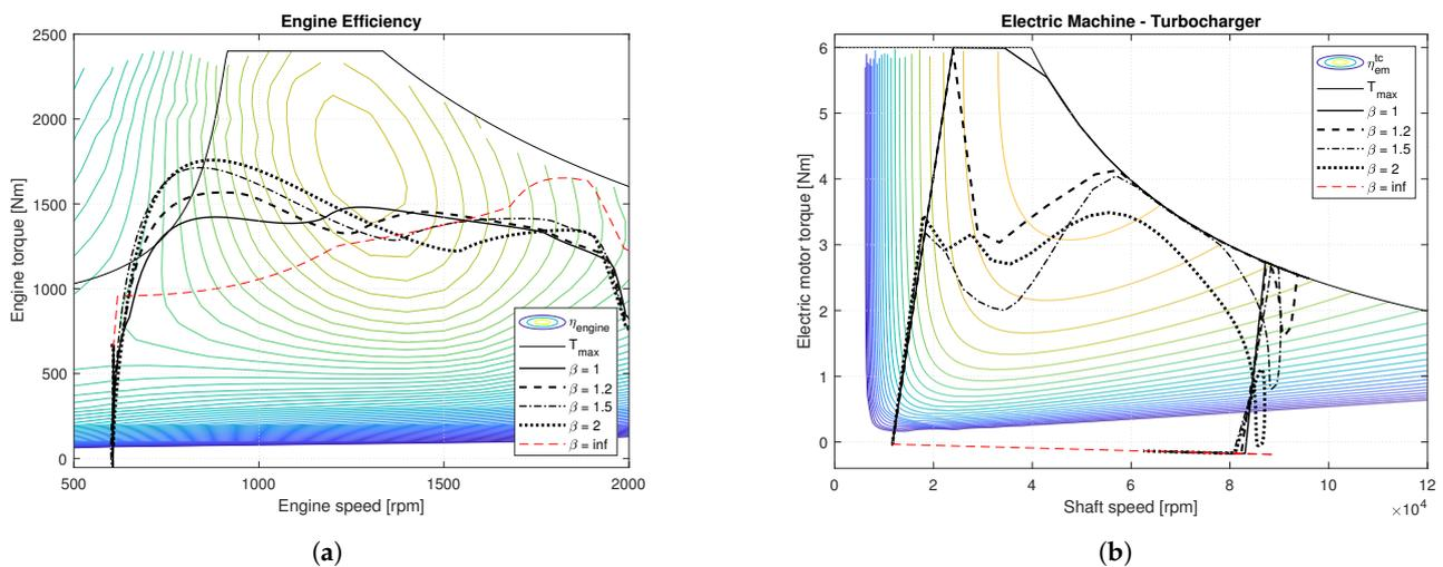
**Figure 7.** Solution characteristics when using a combustion engine and a turbocharged electric motor. The legends display the cost factors ( $\beta$ ) for the different solutions. (a) Diesel engine utilization during an energy-optimal acceleration with E-turbo. (b) Utilization of the E-turbo during the acceleration. When  $\beta = \text{inf}$ , the electric motor torque is negative due to friction.
