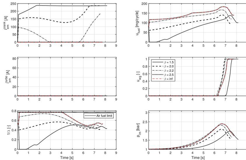
**Figure 10.** Controls, fuel-air ratio and intake manifold pressure during the acceleration when the E-crank is used to support the engine.
