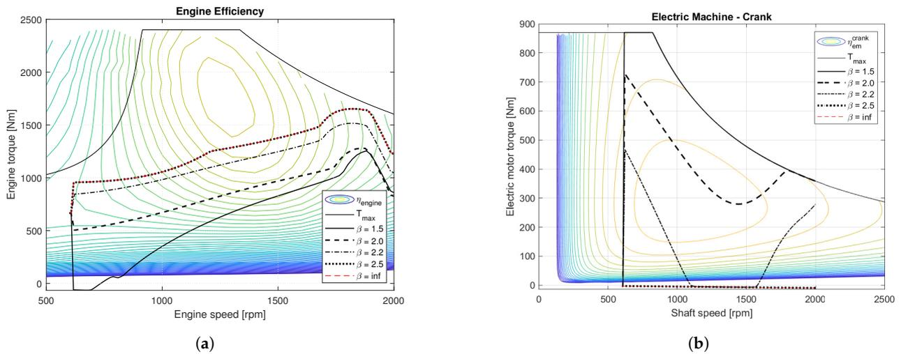
**Figure 9.** Solution characteristics when using a combustion engine and a crank shaft electric motor. The legends display the cost factors ( $\beta$ ) for the different solutions. (a) Diesel engine utilization during a fuel optimal acceleration with E-crank. (b) Utilization of the E-crank during the acceleration. When  $\beta = \text{inf}$ , the electric motor torque is negative due to friction.
