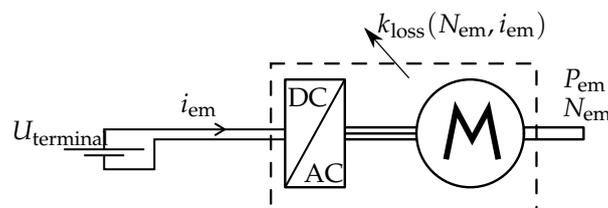
**Figure 3.** Terminology used to describe the electric motor. The dashed line represents the system’s boundary.  $U_{\text{terminal}}$  is the voltage from a constant voltage power supply.
