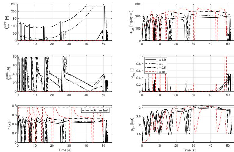
**Figure 13.** Controls, fuel-air ratio and intake manifold pressure during the acceleration from 8 to 80 km/h when both E-crank and E-turbo are used.
