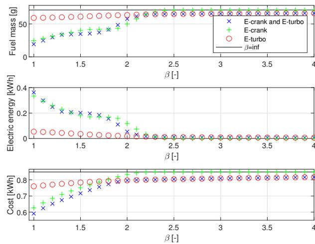
**Figure 6.** Cost factor  $\beta$  in relation to fuel mass consumed (**top**), electrical energy (**middle**) and optimal control cost (**bottom**). An increasing  $\beta$  corresponds to higher cost of electrical energy.  $\beta = \text{inf}$  is the resulting consumed fuel mass if an acceleration is performed without electrical assistance. The cost in the bottom figure is described in (13).
