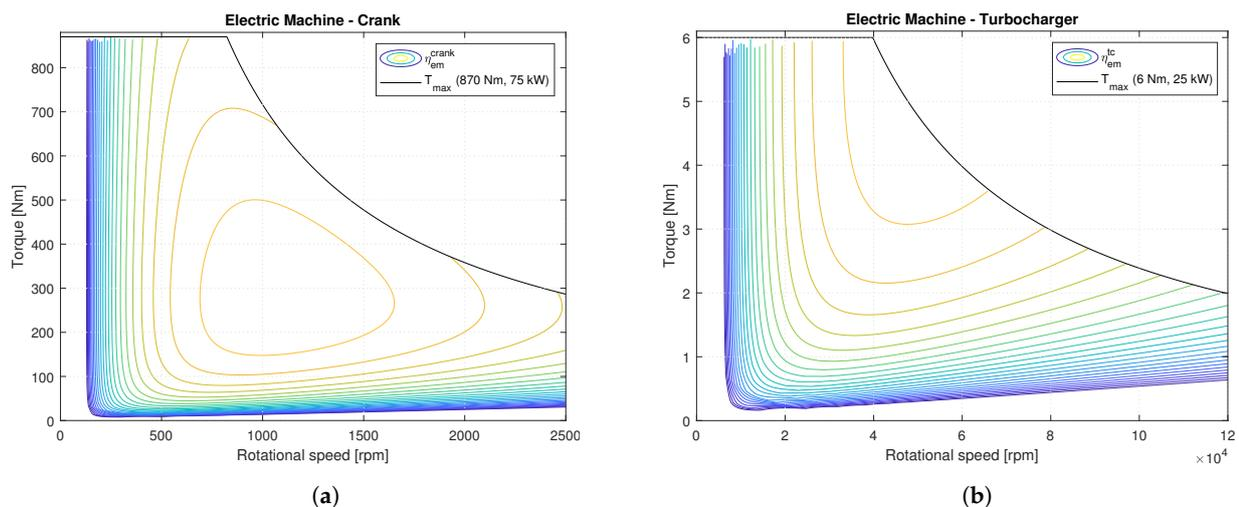
**Figure 5.** Electric motor characteristics for (a) crank shaft motor efficiency lines and the maximum torque restriction, and (b) turbocharger efficiency lines and the maximum torque restriction. The maximum efficiency reached by the combined electric motor and inverter for the two models was 92%.
