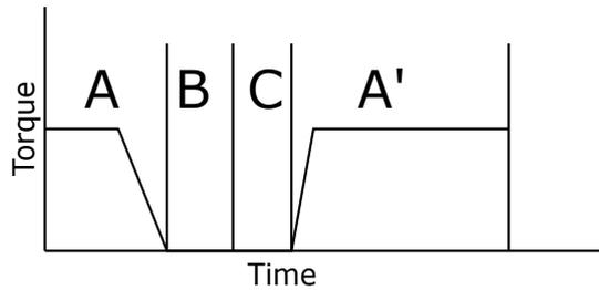
Fig. 5. Example torque demand during a gearshift. The three phases of the gear shift is used as an example to describe how the optimal control models are divided.
