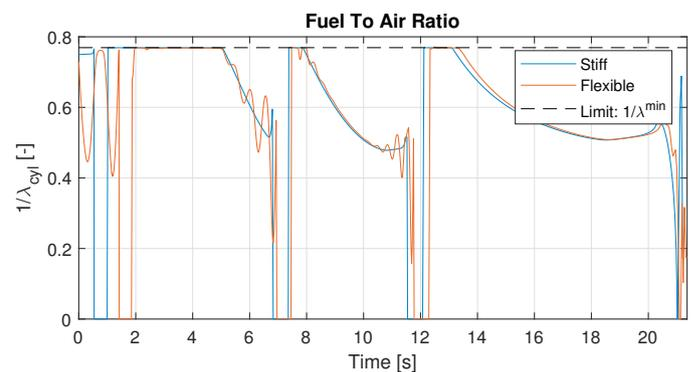
Fig. 10. At the beginning of gear 6, 8, and 10, both the flexible (red) and stiff (blue) driveline are restricted by the fuel to air ratio. There is no way to inject more fuel without producing smoke.
