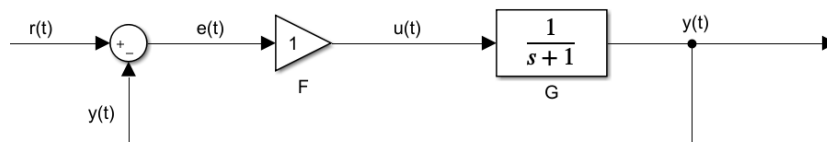
Figure 7: A simple feedback control loop where all names of the signals are displayed where F is the controller and G is an arbitrary transfer function.
