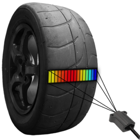
Figure 2.3: Schematic figure of the IRTS sensor [8].
