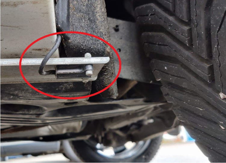
Figure 2.4: Picture of the mounted IRTS sensor.
