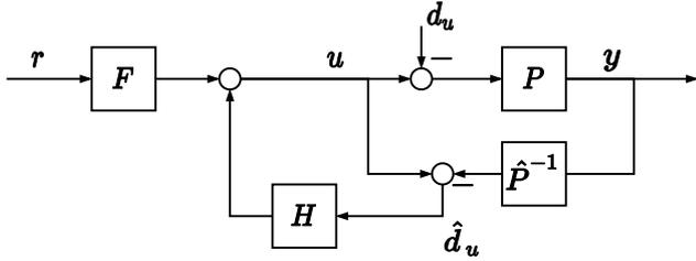
Fig. 5. The disturbance observer controller structure uses the model to estimate an input disturbance  $d_u$ , instead of an output disturbance  $d_y$  like IMC does.
