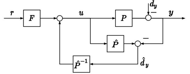
Fig. 6. Ideal IMC, where the estimated output disturbance is fed through an inverse of the model.
