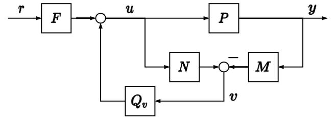
Fig. 8. A general 2-DOF IMC-like controller structure, similar to what Chen (1999) calls the *controller-estimator* or *plant-input-output-feedback* structure.
