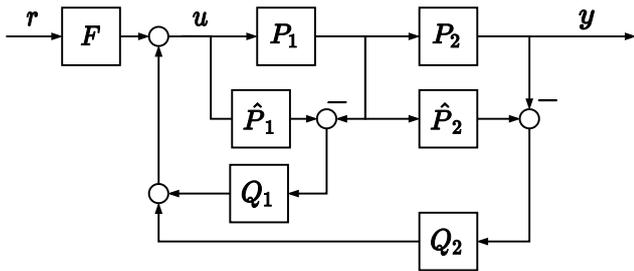
Fig. 16. IMC applied in a cascade control structure.
