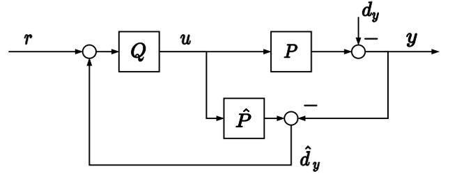
Fig. 2. IMC is often introduced using a 1-degree-of-freedom (1-DOF) structure.
