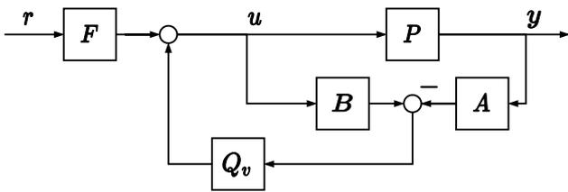
Fig. 9. For a rational SISO system, factorization by the numerator and denominator polynomials yields stable transfer functions.
