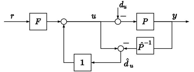
Fig. 7. Ideal DOB, where the estimated input disturbance is cancelled directly.
