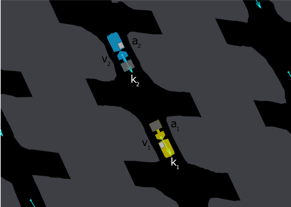
Figure 4.8: An illustration of vehicle orientation. Vehicle v_2 is oriented along its vertex v_2 's vector k_2 meaning its orientation state d(a_2) = 0 . Vehicle v_1 has the opposite meaning d(a_1) = 1 .
