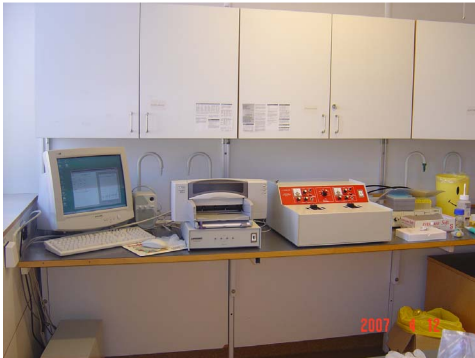
Bild 1 Lumi-aggregometer modell 560-Ca (Chrono-Log Corp., Havertown, PA, USA)
