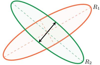
Fig. 1. Covariance ellipses of  $R_1$  and  $R_2$  corresponding to  $y_1$  and  $y_2$ , respectively. An optimal scalar subspace to project  $y_2$  onto is likely given by a vector approximately aligned with the minor axis of the  $R_2$  ellipse, illustrated by the black arrow.
