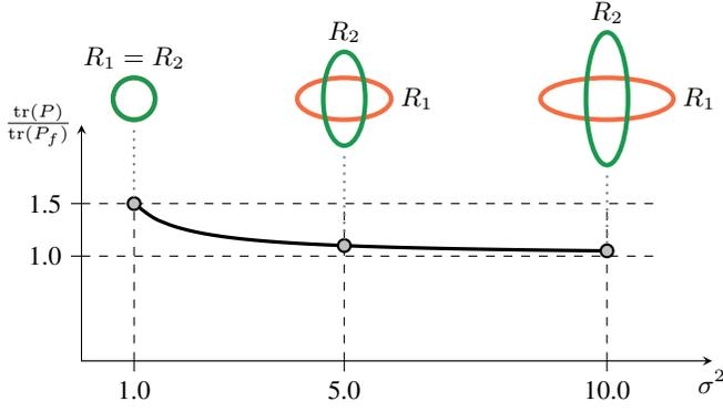
Fig. 2. The ratio  $\frac{\text{tr}(P)}{\text{tr}(P_f)}$  indicates that using  $y_\Psi$  instead of  $y_2$  does not significantly reduce the performance in many cases. The ellipses of  $R_1$  and  $R_2$  corresponding to  $\sigma^2 = 1.0$ ,  $\sigma^2 = 5.0$  and  $\sigma^2 = 10.0$  are shown in the top.
