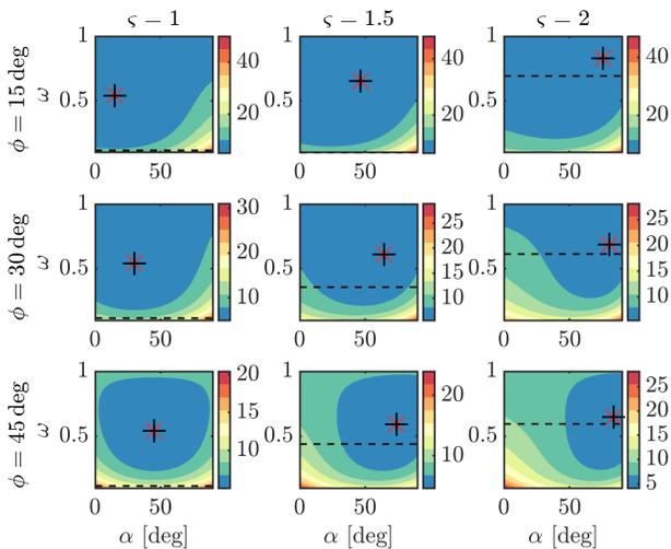
Fig. 7. Each row and column correspond to one value of  $\zeta$  and  $\phi$ , respectively. The red cross and the black plus sign correspond to an optimal  $\Psi$  found by a grid search and as computed by Algorithm 1, respectively. The dashed black line resembles  $\omega$  given by step 1 of Algorithm 1.
