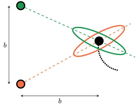
Fig. 8. Simulated scenario. The green and the orange circles are stationary agents that track a common target (black circle) by observing, filtering and exchanging estimates of the target. The ellipses centered at the target represents 95% confidence ellipses of the measurement covariance  $R_k^S$  in each agent. The target moves along the dotted curve.
