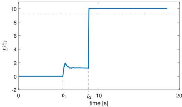
Fig. 4. The hypothesis score  $L^{\mathcal{H}}_{s_1}$  for the landmarks in group  $s_1$  in Fig. 3. At  $t = t_1$  the hypothesis score is initialized and at  $t = t_2$  also the single hypothesis landmark in group  $s_2$  comes into field-of-view increasing the probability of  $\delta^1 = 1$ . The dashed line marks the threshold in the SPRT test.
