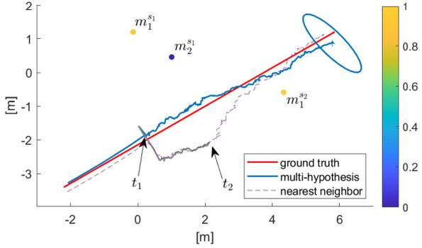
Fig. 3. The blue line shows the estimated trajectory with the uncertainty ellipse at the final time step, the red line is the true trajectory and the grey line is the rejected hypothesis. The purple dashed line is the nearest neighbor trajectory estimate. Landmarks are marked with colored dots where the colorbar indicates the estimated probability of existence of the landmarks at the final time step.
