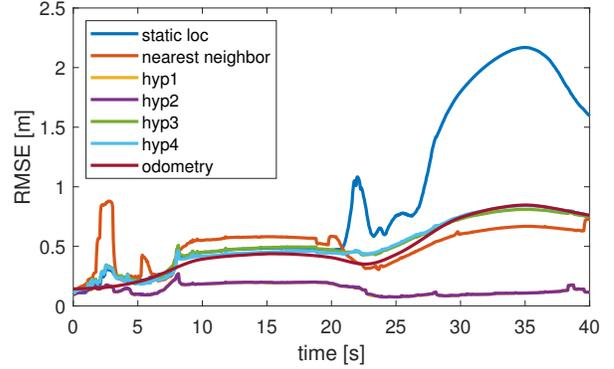
Fig. 5. The RMSE of 1000 MC realizations of the trajectory state estimation. Results are given for four different utilization levels of the map uncertainty when adopting the multi-hypothesis map representation. Also the results of a static localization assuming all doors are always opened, a nearest neighbor solution, and a pure odometric dead-reckoning localization are presented. (Note that *hyp1* is almost completely hidden by *hyp2*.)
