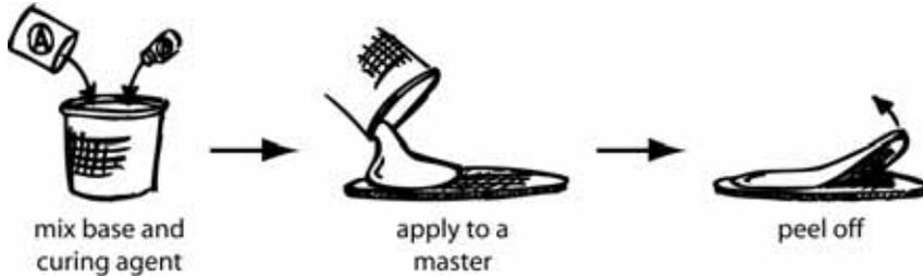
**Figure 4.4:** The basic steps for PDMS stamp fabrication.
