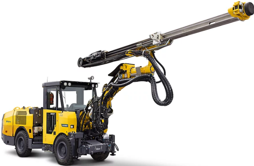
Figure 1.1: Drill rig with one boomer.
