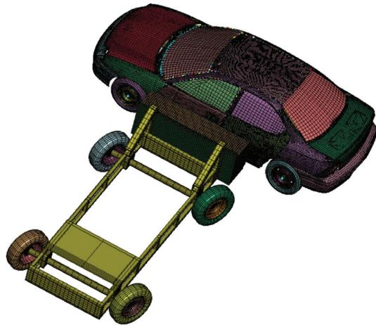
**Figure 14:** The car crashworthiness design problem: car finite element model diagram (Yildiz et al., 2021).
