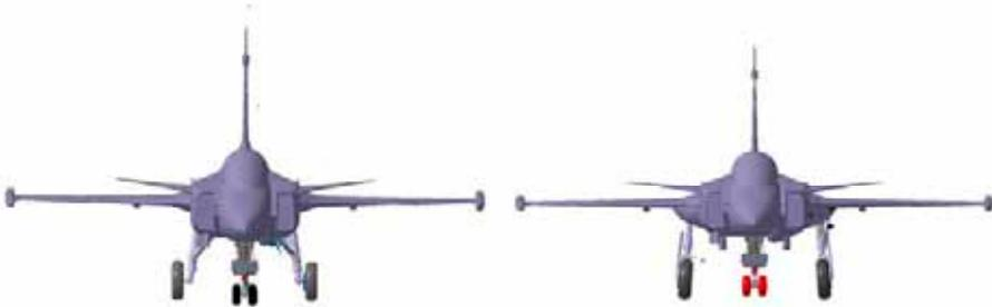
Figure 19: *The present (left) and proposed new (right) landing gear.*
