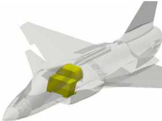
Figure 16: *The forward fuselage section of the two-seater mounted on a single seat a/c, and with the aft seat replaced with a fuel tank.*
