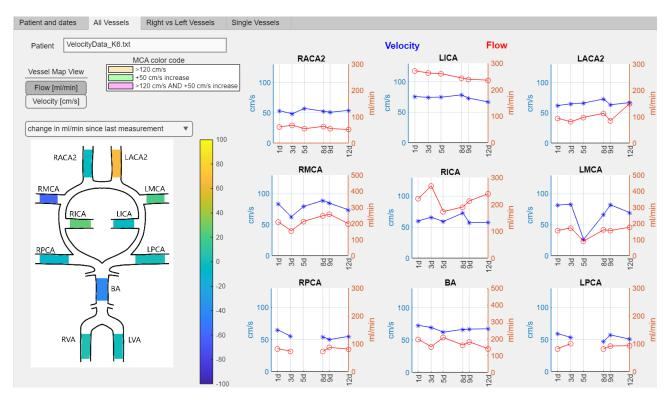
Figure 4.10: First view of the second tab, containing a 2D generic vessel map along with a nine plot setup of flow and maximum velocity visualization.
