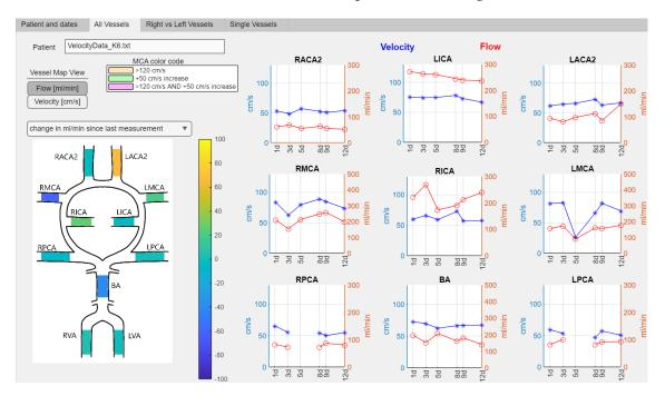
Figure 7.4: First view of the second tab, containing a 2D generic vessel map along with a nine plot setup of flow and maximum velocity visualization.
