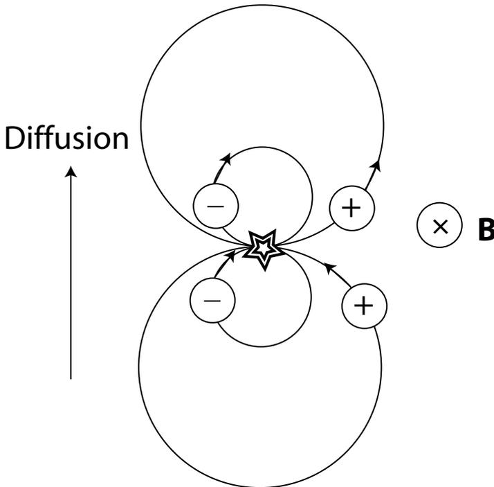
Figure 9. Collision between an electron and an ion resulting in a shift of the guiding centers and a cross-field diffusion. The magnetic field line is here directed into the plane of the paper. (After F.F. Chen [17].)
