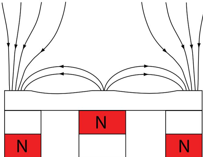
**Figure 14.** Schematic drawing of a cross section of an unbalanced magnetron, displaying the magnetic field lines as only partially closed loops above the target surface. Here, the electrons can more easily escape and travel towards the substrate region.
