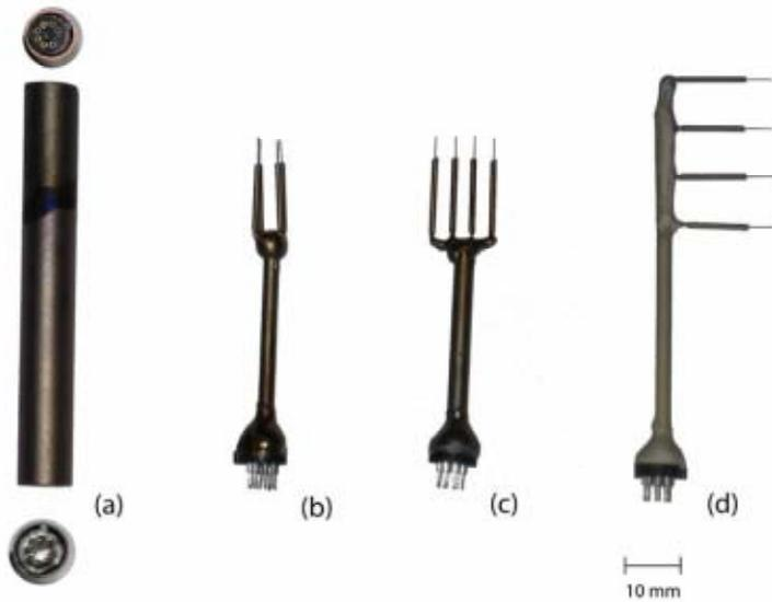
**Figure 11. Electric field probes and transformer used for measuring oscillations. (a) Impedance matching unit with connector sides. (b) Four-pin probe measuring  $E_\rho$  and  $E_\phi$ . The distance between the probe tips is 6 mm. (c) Fork-probe measuring azimuthal phase velocity,  $v_\phi$ . The distance between the probe tips is 4 mm. (d) Probe measuring  $E_z$  oscillations. The distance between the probe tips is 10 mm.**
