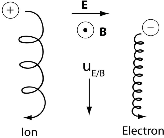
**Figure 6.** Single particle motion in combined electric and magnetic fields.  $\mathbf{B}$  points out of the plane of the paper. (After F. F. Chen [15].)
