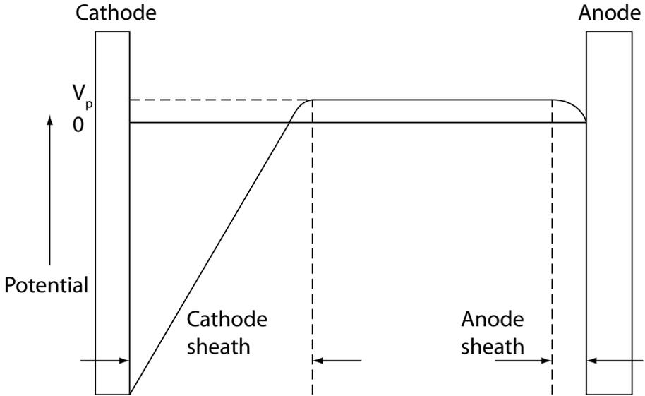
**Figure 4. Potential distribution from a dc discharge. Here the cathode is the negatively biased magnetron and the anode is the chamber walls.  $V_p$  is the plasma potential. The fall in potential is indicated for each sheath region. (From M. Ohring [6].)**
