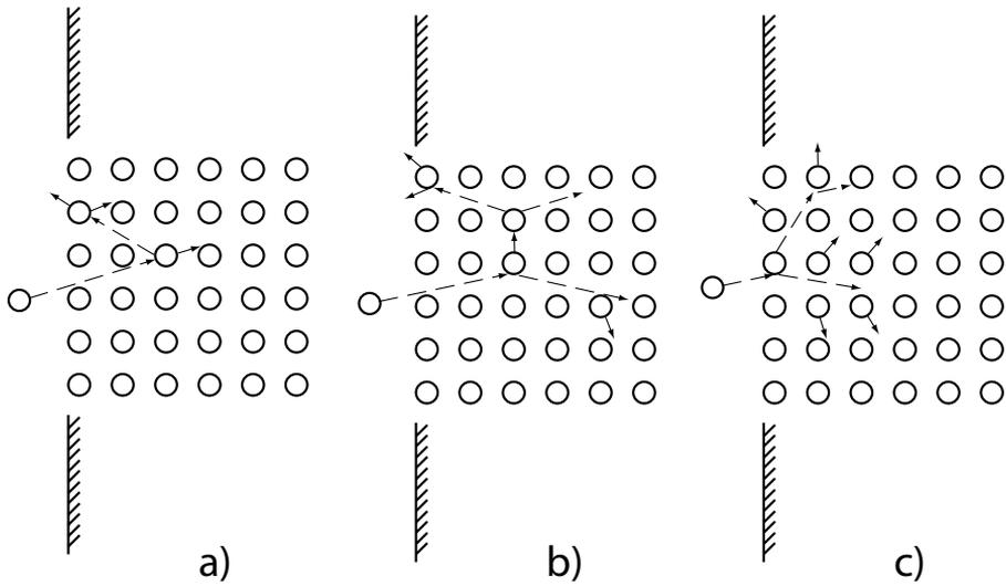
**Figure 5. Energy regimes of sputtering: a) Single knock-on (low energy), b) linear cascade, and c) spike (high energy). (After P. Sigmund [18].)**
