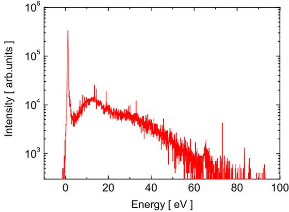
**Figure 3. Time-averaged  $\text{Ti}^+$  ion energy distribution in a HIPIMS discharge.**
