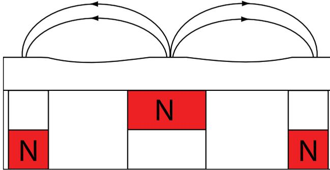
**Figure 13.** Schematic drawing of a cross section of a balanced magnetron, displaying the magnetic field lines as closed loops above the target surface. Between the inner and outer magnetic rings the target displays an erosion track, or the so-called race track.
