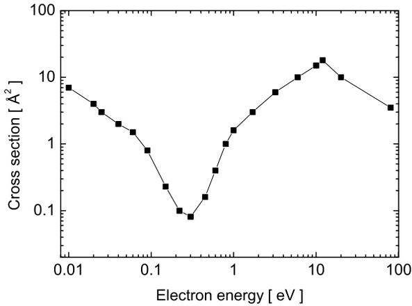
**Figure 8. Momentum transfer cross section for argon, showing the so-called Ramsauer minimum. (After [17, 20].)**
