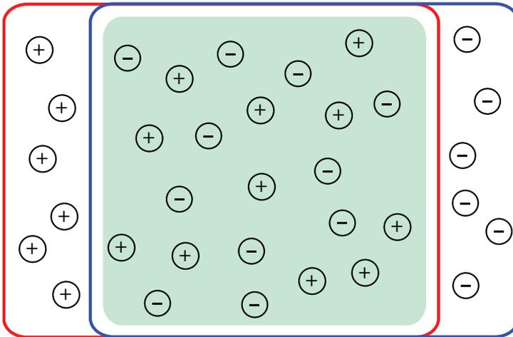
**Figure 7. Electron cloud slightly displaced from the cloud of positive ions. In the middle the quasineutral plasma.**
