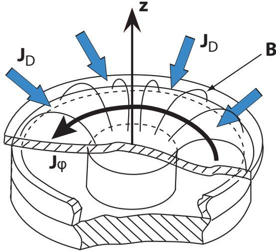
**Figure 12. A circular planar magnetron cathode, showing the shape of the magnetic field, the current densities and the resulting drift path.**
