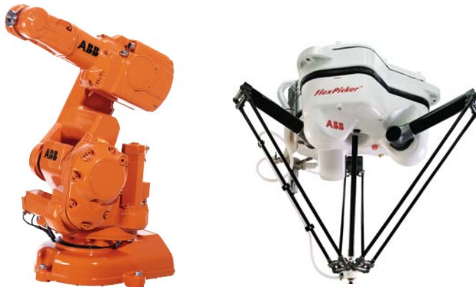
Figure 2.1 On the left, an ABB IRB 140, which is an articulated robot with an open kinematic chain. On the right, an ABB Flexpicker robot, which is a parallel robot consisting of closed kinematic loops.
