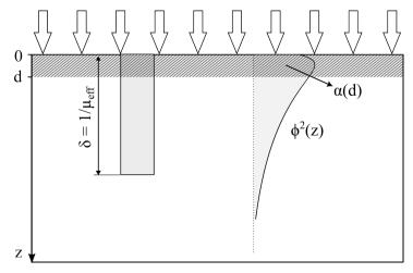
Figure 5.1: Geometry of the model. The top layer of thickness d has a scattering coefficient  $\mu'_{s,top}$ , and the bottom layer has a scattering coefficient  $\mu'_{s,bot}$ . On the left, is shown the linear partial volume contribution, given by  $d/\delta$ . On the right is the fluence integral partial volume contribution  $\alpha(d)$ .
