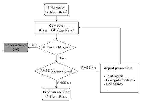
Figure 5.2: Flowchart of the inverse solving algorithm
