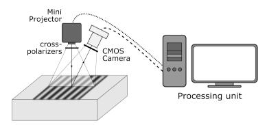
Figure 3.2: Schematic of a typical SFDI system
