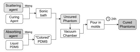
Figure 4.2: A chart of the process for fabricating silicone phantoms.
