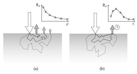
Figure 3.1: Monte Carlo simulations of diffuse reflectance ( $R_d$ ) in the space domain (a) and in the time domain (b).
