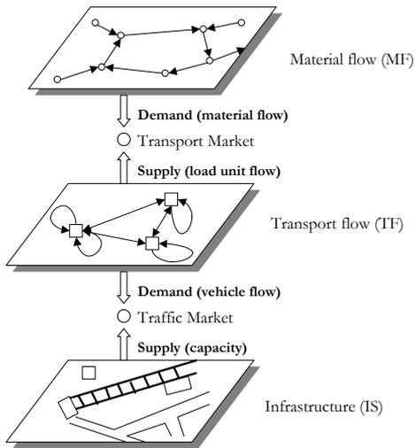
**Figure 5: Model relating different levels of transport (Wandel et al, 1992, p 98)**
