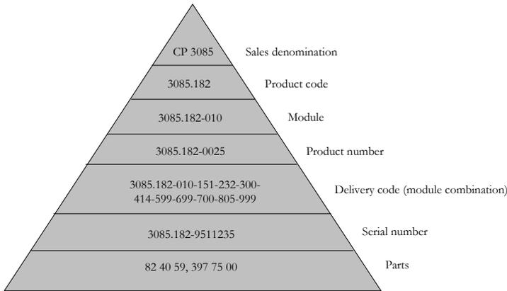
**Figure 24: Example of the ITT Flygt "Identity pyramid"**
