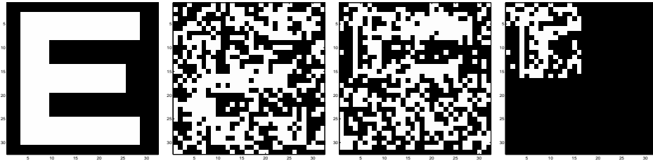
Figure 5.11: Embedding type 1. (a) Binary watermark image. (b) After attack with noise. (c) After attack with edit. (d) After attack with cropping.
