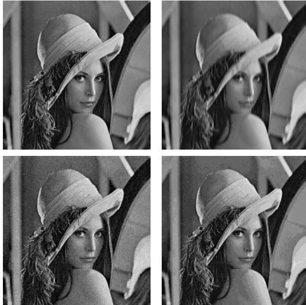
Figure 2.2: (a) Original Lenna image (b) Image attacked with low-pass filter. (c) Image attacked with Gaussian noise. (d) Image attacked with quantization.
