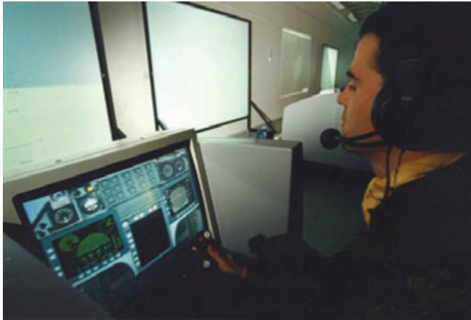
Figure 12. One of the pilot stations of FLSC with the layout from the time of the study 17 . Other pilot stations and the exercise manager's "God's Eye presentation" can be seen in the background. During the study covers were drawn between the pilot stations.
