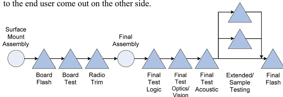
**Figure 6:** Typical production and test flow.
