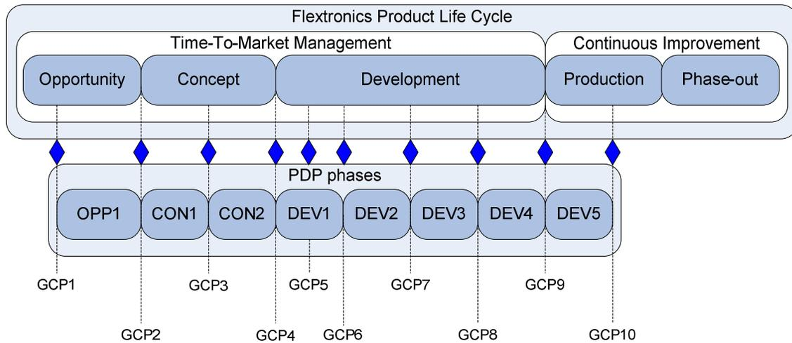
**Figure 8:** The interconnection between the phases in the FPLC and the PDP.
