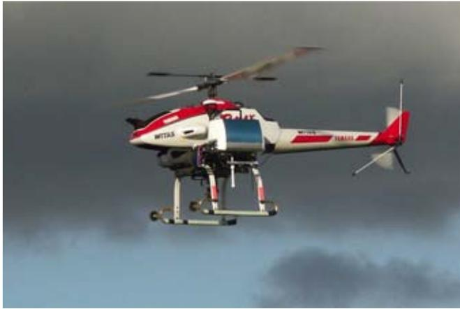
Figure 1.1: The Yamaha RMAX helicopter.
