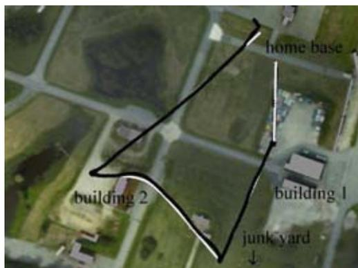
Figure 8.1: An interactive mission visiting a number of locations in the flight-test area in Revinge. The planned paths are white and the logged data from the flight is black.
