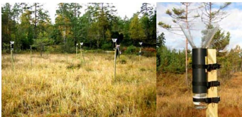
**Figure 3.** Precipitation sampling at Stubbetorp. Nine collectors were placed at least 3.5 m apart and at a height of 160 cm. (photo: Frank Laturmus)
