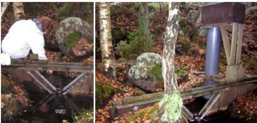
**Figure 4.** Runoff sampling for Papers II and III at the spring, where the water discharge was measured by a V-notch weir with a gauge (in the box at the right picture) measuring the water table. (photo: Teresia Svensson)
