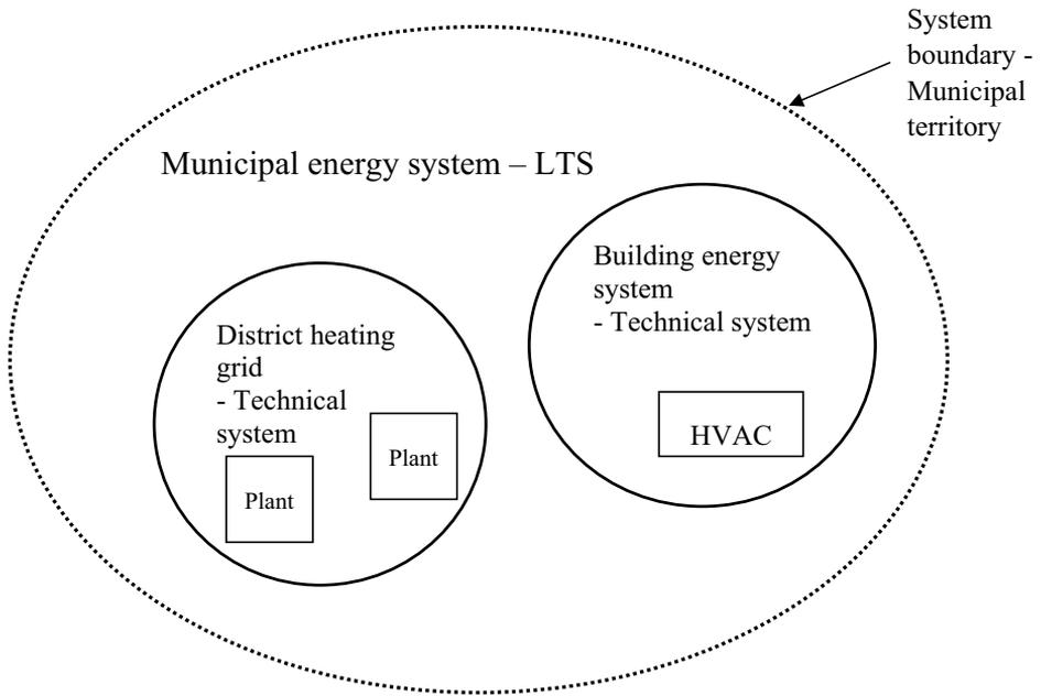
Figure 1. A municipal energy system with part systems on detailed level (boxes) and technical systems level (circles).
