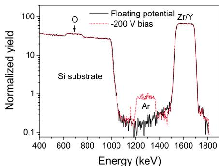
FIG. 4. (Color online) Log-scale plot of the RBS spectra from two YSZ films on Si deposited at 400 °C for 30 min at a floating substrate bias potential and a substrate bias of  $-200$  V, respectively. An Ar impurity content of 1.5 at. % is observed in the  $-200$  V film.
