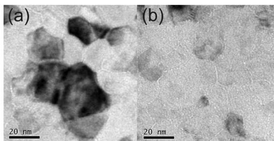
FIG. 5. Underfocused (bright-field) TEM images of the samples deposited at biases of (a)  $-150$  and (b)  $-200$  V. The picture in (b) shows a large quantity of tiny white dots, which are interpreted as small Ar bubbles.
