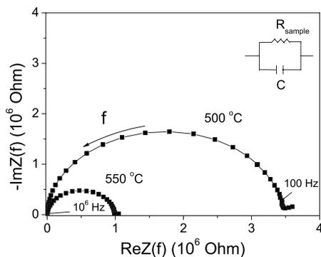
FIG. 7. Typical impedance spectra measured at 500 and 550 °C for a film with thickness  $d=1\ \mu\text{m}$  deposited on quartz at 400 °C with a bias of  $-70\ \text{V}$ . The frequency range used was 1 MHz–42 Hz.
