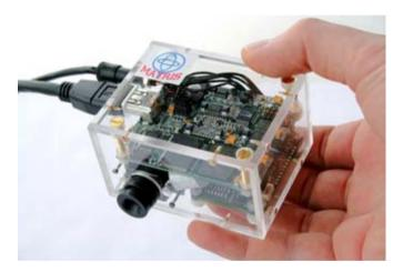
**Figure 1.7:** This is a prototype developed in the MATRIS project. It consists of a camera, an IMU and a low-power digital signal processor, used for pre-processing of the sensor signals. Courtesy of Xsens Technologies B.V.
