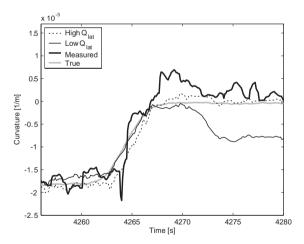
**Figure 1.3:** Comparison of estimation performance from two filters, one with a large  $Q_{lat}$  and one with a small  $Q_{lat}$ . The raw measurement signal from the image processing unit is also included. Comparing this raw vision measurement to the result from the filters clearly illustrates the power of a model based sensor fusion approach.
