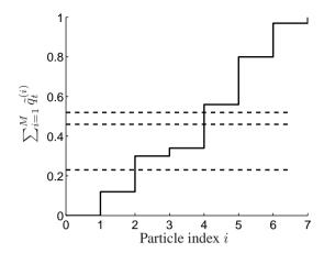
**Figure 4.1:** Illustrating the resampling step in the particle filter. The new set of particles is obtained by first generating M sorted uniformly distributed random numbers, three of which are shown by the dashed lines in the figure. These are then associated with a particle guided by the cumulative sum of the normalized importance weights. In the figure particle number 2 is chosen once and particle number 4 is chosen twice.
