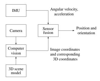
**Figure 1.6:** Schematic illustration of the approach. The sensor fusion module is basically a recursive nonlinear state estimator, using information from the inertial measurement unit (IMU) and the computer vision system to compute an estimate of the position and orientation of the camera.
