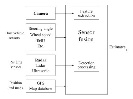
**Figure 1.1:** The most important factor enabling future automotive safety systems is the availability of accurate information about the state. The process of obtaining this information is to a large extent dependent on a unified treatment of the sensor information, as illustrated in this figure. The aim of this sensor fusion approach is to provide the best information possible for as many purposes as possible. In Section 1.2 this strategy is exemplified using the sensors in bold font.
