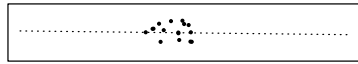
Figure 3.5. A bad set of points with low cost when fitting a straight line
