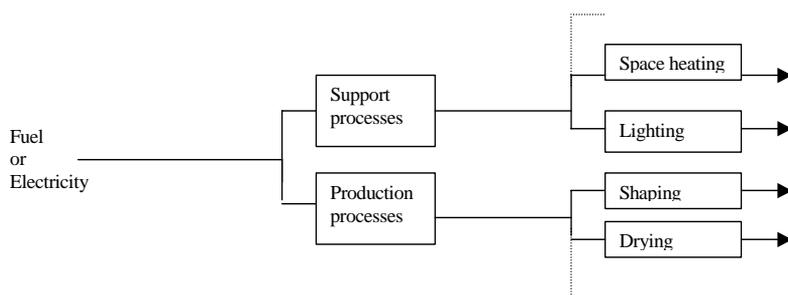
*Figure 10: Example of energy flows divided into support and production processes*
