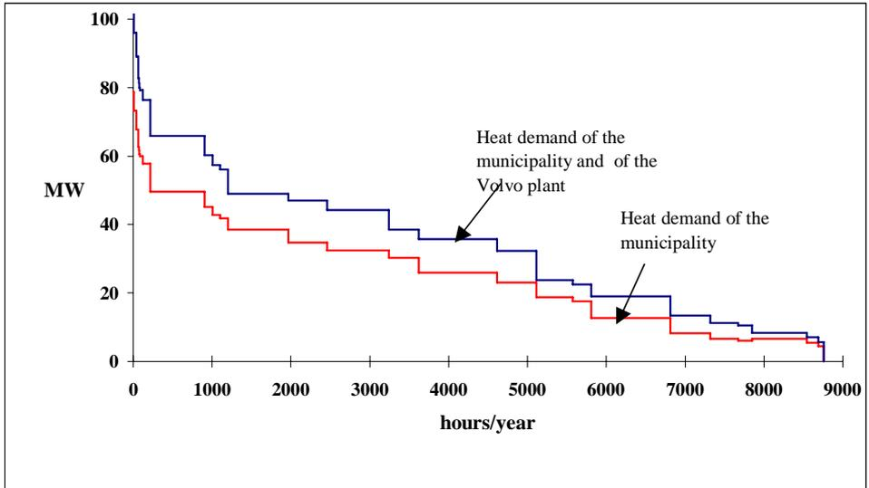
Figure 22: Load duration curves for district heating before and after the Volvo plant converts hot tap water, space heating and cooling to district heating.
