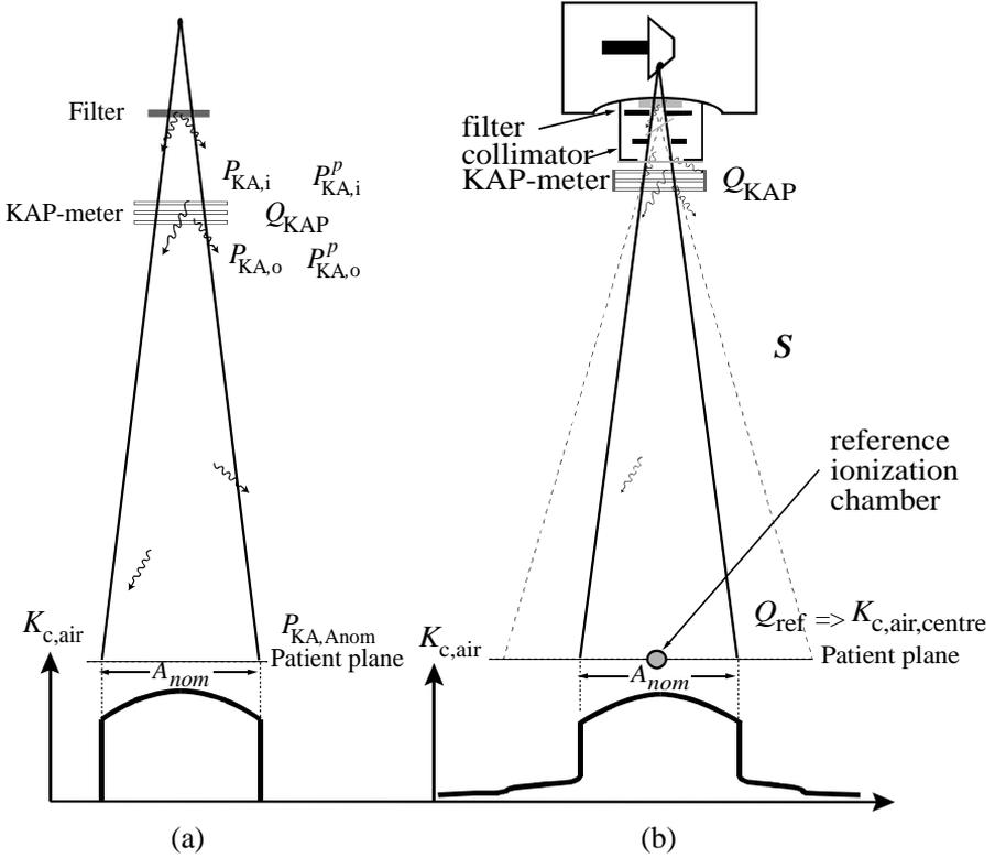
Figure 14. (a) The geometry of the Monte Carlo simulations and quantities derived using these simulations. (b) The measurement geometry and quantities derived.
