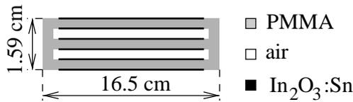
Figure 16. Schematic side view of the KM3. The quadratic surface area of the KAP-meter is 165 mm x 165 mm. The size and construction of KM1 and KM3 are similar, see the text for details (from Paper V).
