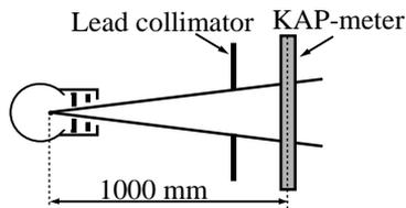
Figure 2. Schematic view of the experimental set-up for the calibration of a Master KAP-meter using a collimator with a well-defined aperture to determine the beam area. The KAP-meter signal is related to the air kerma area product of the incident photons as measured at a standard laboratory using a free-air chamber (from Paper V).
