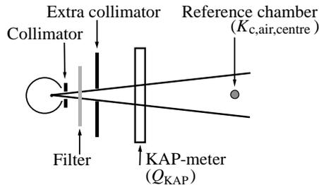
Figure 17. Experimental set-up for measuring the sensitivity (see text for explanation). The housing for the adjustable collimators was replaced with a single lead collimator (5 mm thick) with a circular aperture with diameter 30 mm. The filter, collimator, KAP-meter and reference chamber were placed 6, 11.8, 30 and 110 cm respectively from the focal spot.
