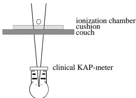
Figure 12. Geometry at under-couch calibrations.
