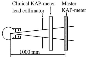
Figure 8. Calibration of a clinical KAP-meter using a Master KAP-meter.
